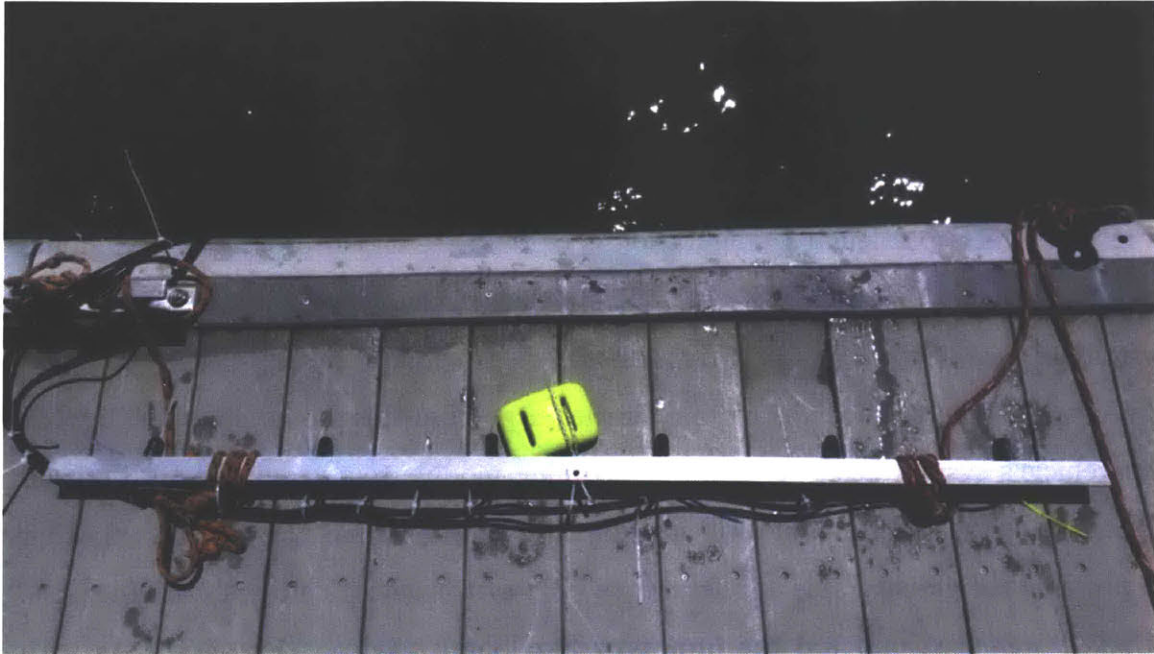
Figure 4-1: Line array with 6 channels and adjustable spacing.
