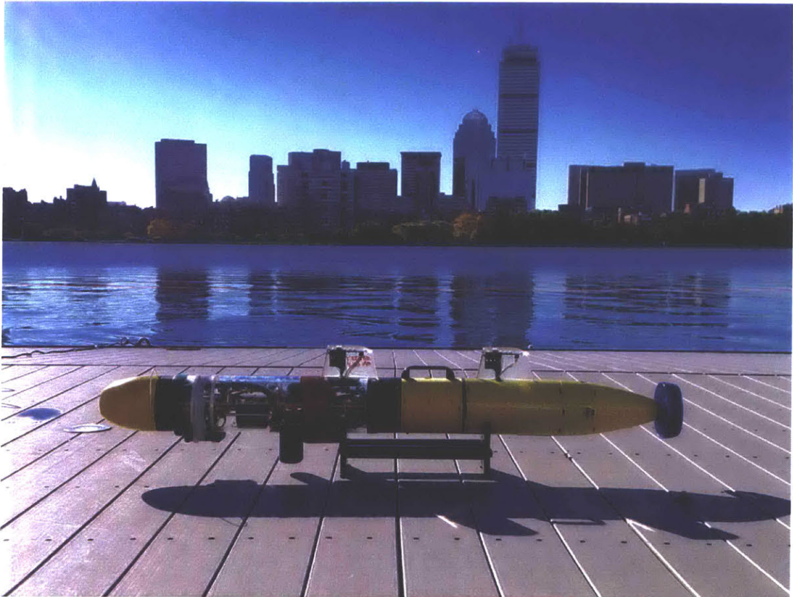
Figure 4-7: SandShark AUV, during preparations for deployment in the Charles River Basin to perform behavior-triggering experiments.
