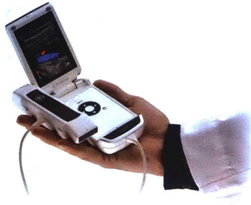
Figure 1-1: Vscan™: General Electric's handheld, pocket-sized ultrasound tool [1].
