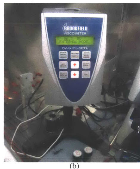
Figure 4.6.1 (a) Schematic of a section through the testing device used for conductivity measurements. The electrodes were made out of stainless steel, while the rest of the device was constructed out of PVDF for chemical and mechanical stability. (b) Picture of the digital viscometer used in rheological measurements inside the Ar-filled glove box.
