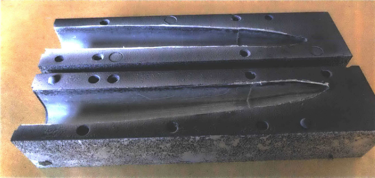
Figure 100: The front quarters of the propellant mold, coated with release agent (black) and containing the inhibitor shells (white).
