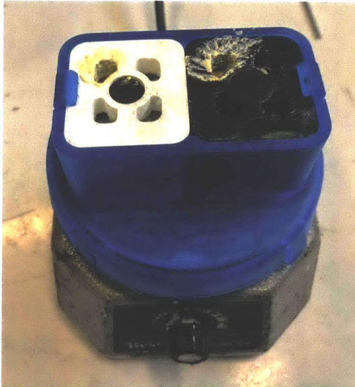
Figure 124: Two nozzle molds are mounted on a vibrating platform and filled with ceramic slurry.
