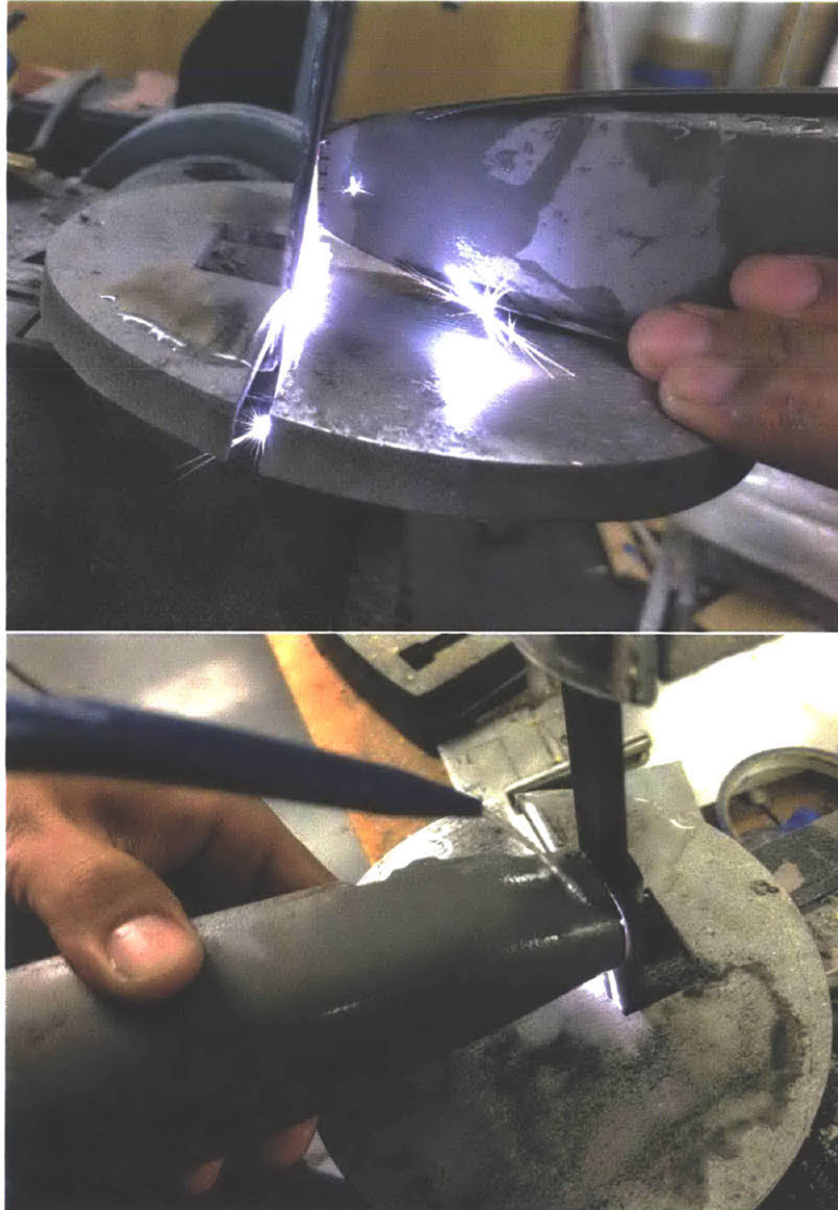
Figure 87: A belt sander is used to remove support material from the part. Water cooling is required to prevent overheating because of titanium's poor thermal conductivity.
