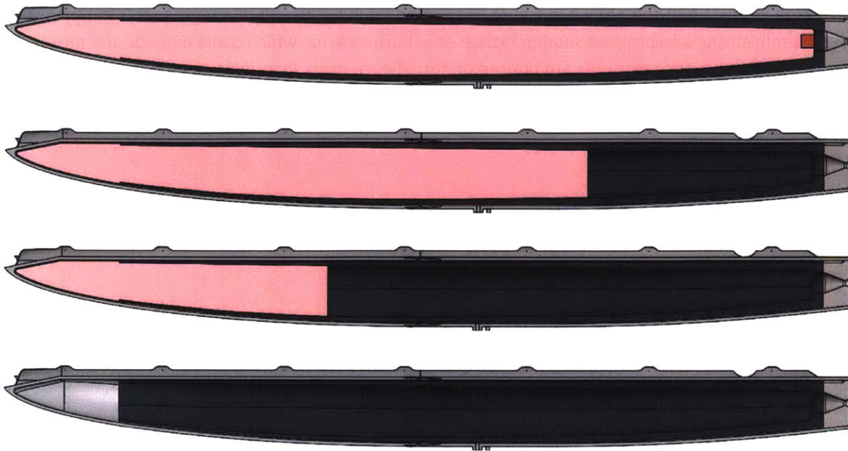
Figure 53: Evolution of the end-burning propellant grain during the burn.
