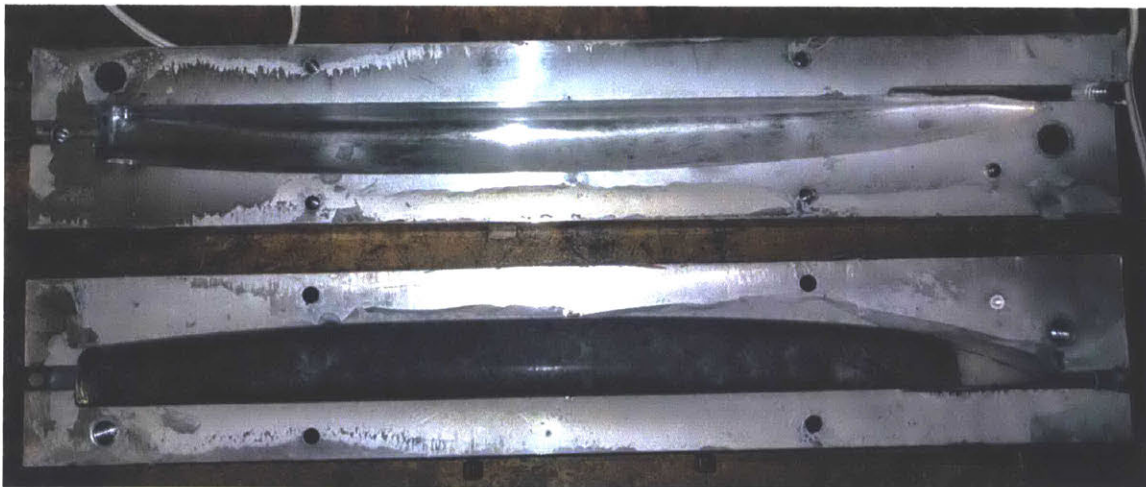
Figure 112: The open liner mold reveals the cured liner and propellant inside.
