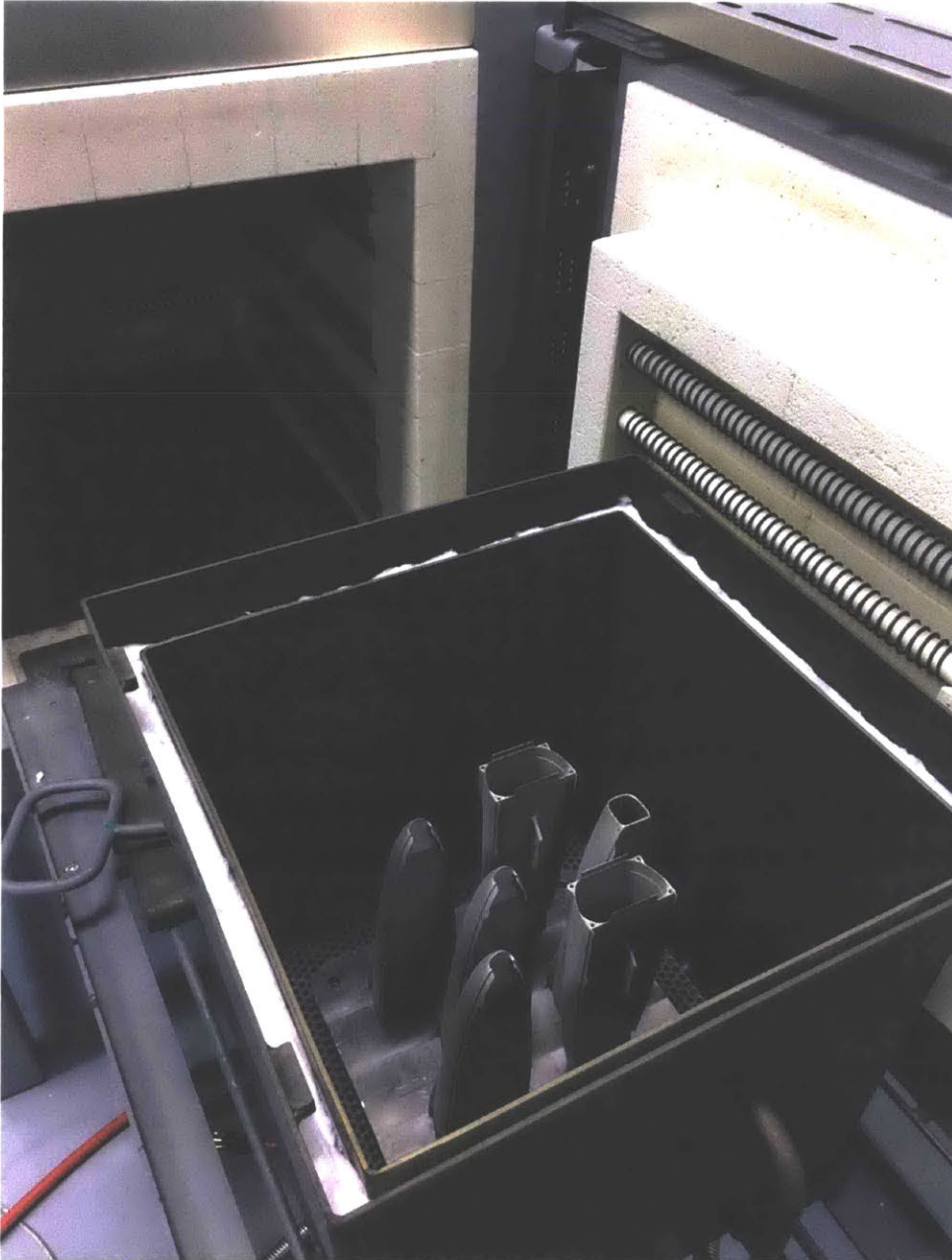
Figure 85: Motor case parts are loaded into a gas-tight chamber and placed in a furnace for heat treatment. Photo credit Renishaw plc [69].
