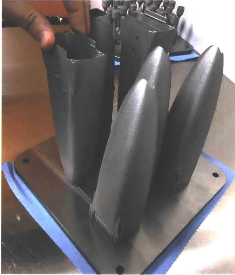
Figure 84: Near net shape parts emerge from the printer welded to a build platform by support material. Photo credit Renishaw plc [69].
