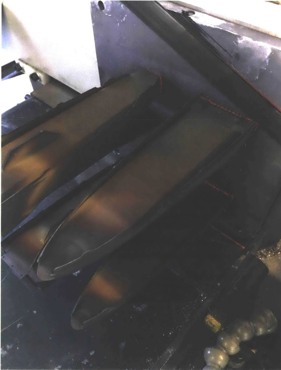
Figure 86: A saw cuts through support material to remove the parts from the build platform. Photo credit Renishaw plc [69].
