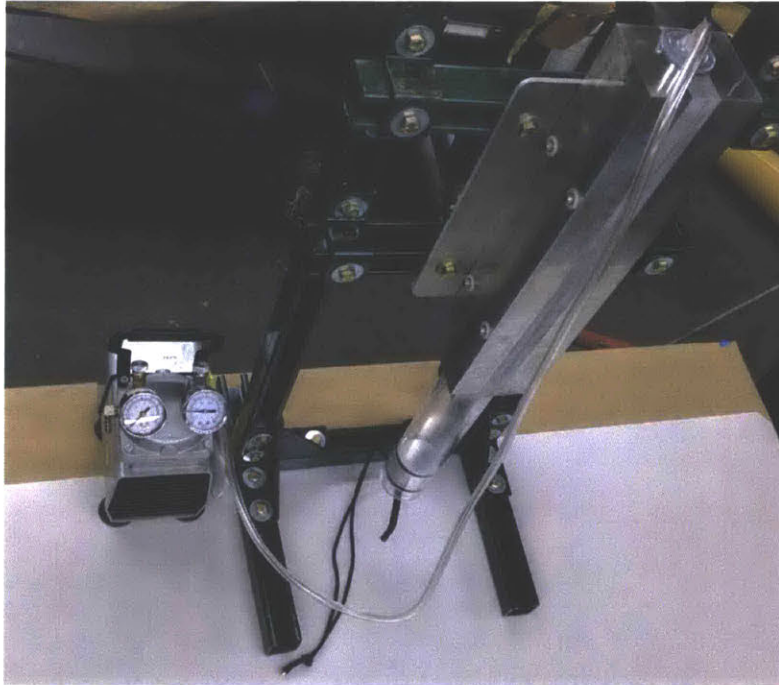
Figure 110: The assembled liner mold mounted on its stand.
