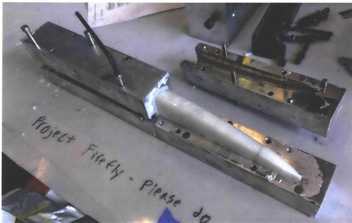
Figure 103: The propellant mold is opened using the parting screws. This photo was taken during a pathfinder casting with inert propellant; the propellant is white to signal that it is inert.
