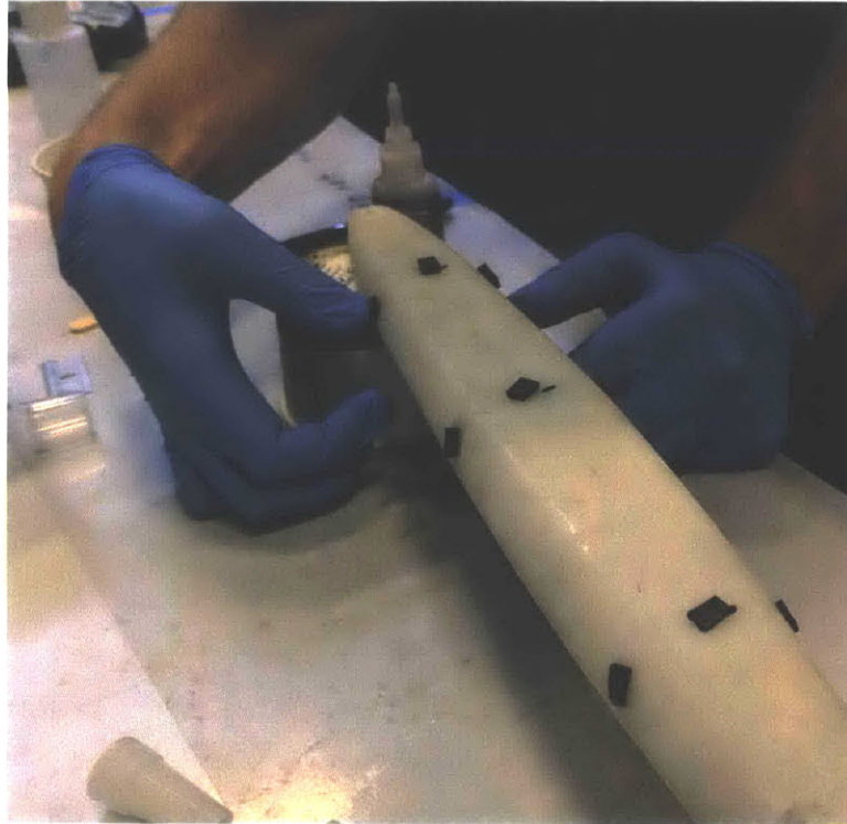
Figure 105: Applying shims to a propellant grain in preparation for liner casting. This photo was taken during a pathfinder casting with inert propellant; the propellant is white to signal that it is inert.
