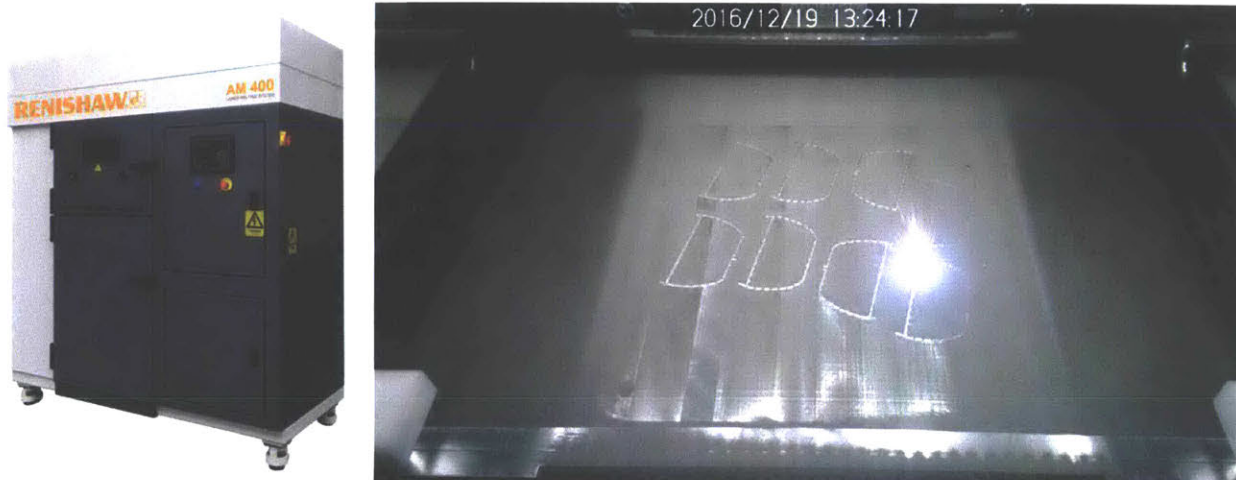
Figure 83: Left, the Renishaw AM400 printer. Right, the printer's laser fuses a Firefly motor case prototype. Photo credit Renishaw plc [69].
