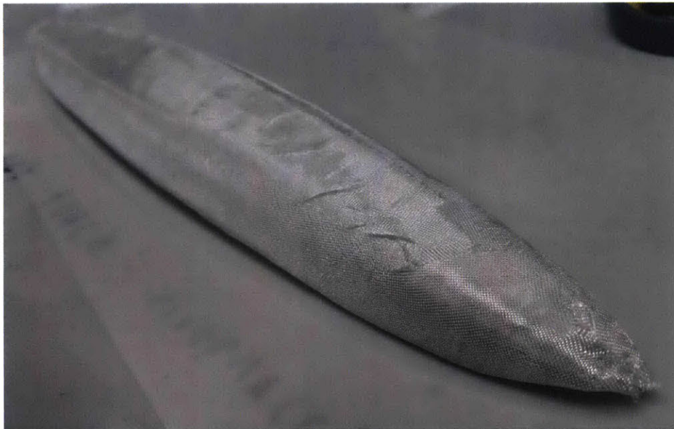
Figure 120: The finished propellant package, with fibrous insulation wrapped around the propellant and liner.
