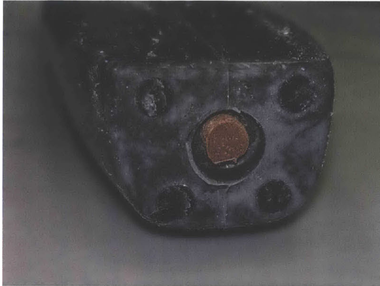
Figure 115: A starter grain (brown-red, center of image) after installation.
