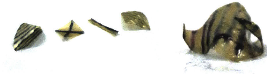
Figure 7-9. Example of anthocyanin at pH 10 solution patterned on shape changing material to induce shape-color change
