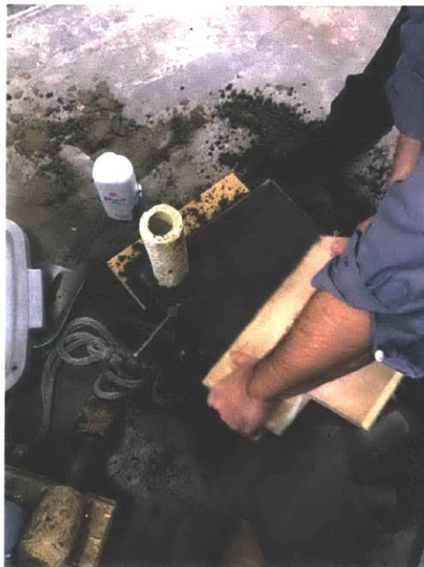
Figure 45: Flat board was used to remove excess sand and achieve a flat surface on mold
