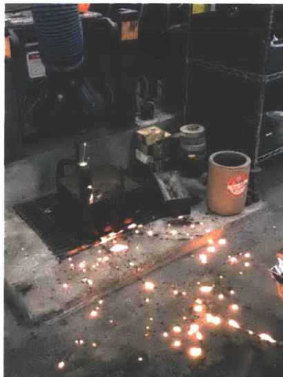
Figure 54: Aftermath of sprue exploding
