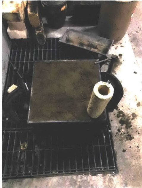
Figure 51: Mold clamped shut and ready for pouring
