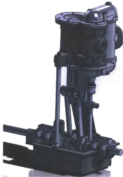
Figure 8: Assembly CAD for the 3 ½ by 3 ½ circulating steam engine
