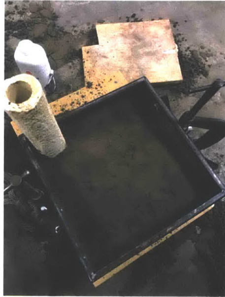
Figure 44: The sprue was added and green sand was used to pack the rest of the mold
