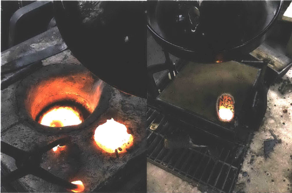
Figures 52 & 53: Metal being melted and mold after metal being poured through the sprue
