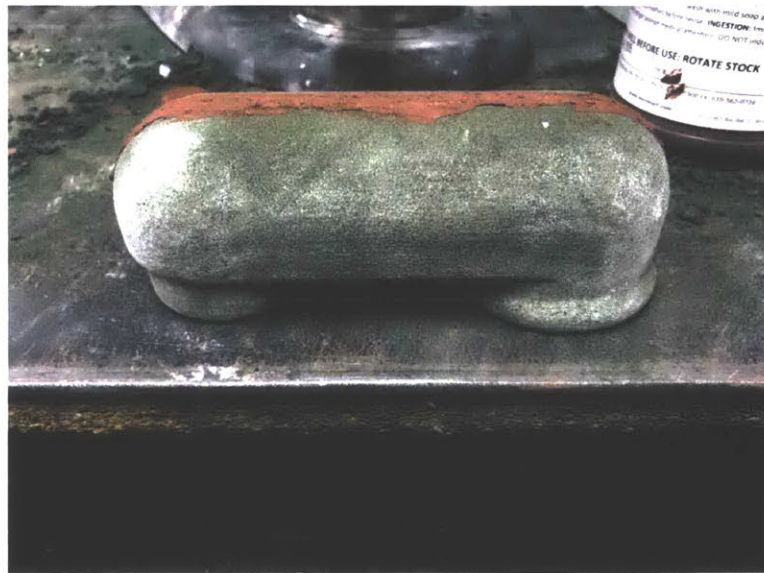
Figure 36: Two core halves glued together using an acetone based adhesive
