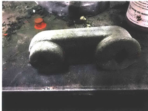
Figure 30: Core halves are glued together using an acetone based adhesive
