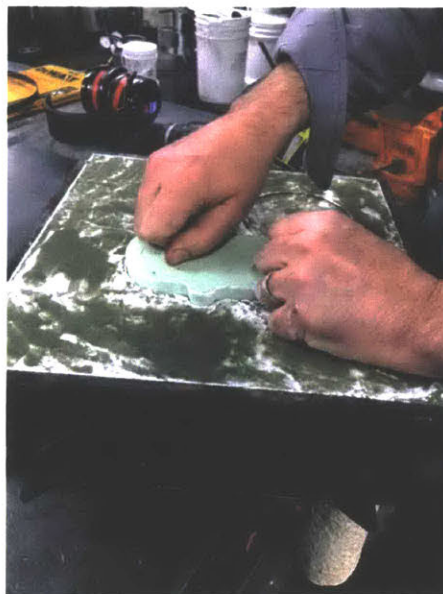
Figure 48: Pattern was removed from mold using screws
