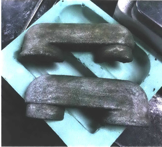
Figure 35: Core halves after being removed from core mold
