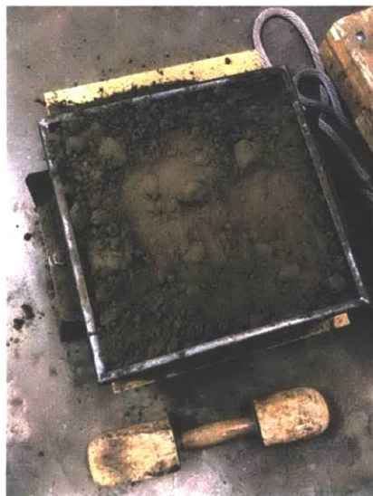
Figure 41: Rammer is used to pack sand tightly
