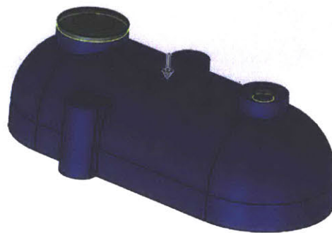
Figures 12 & 13: Holes and hollow areas are filled in
