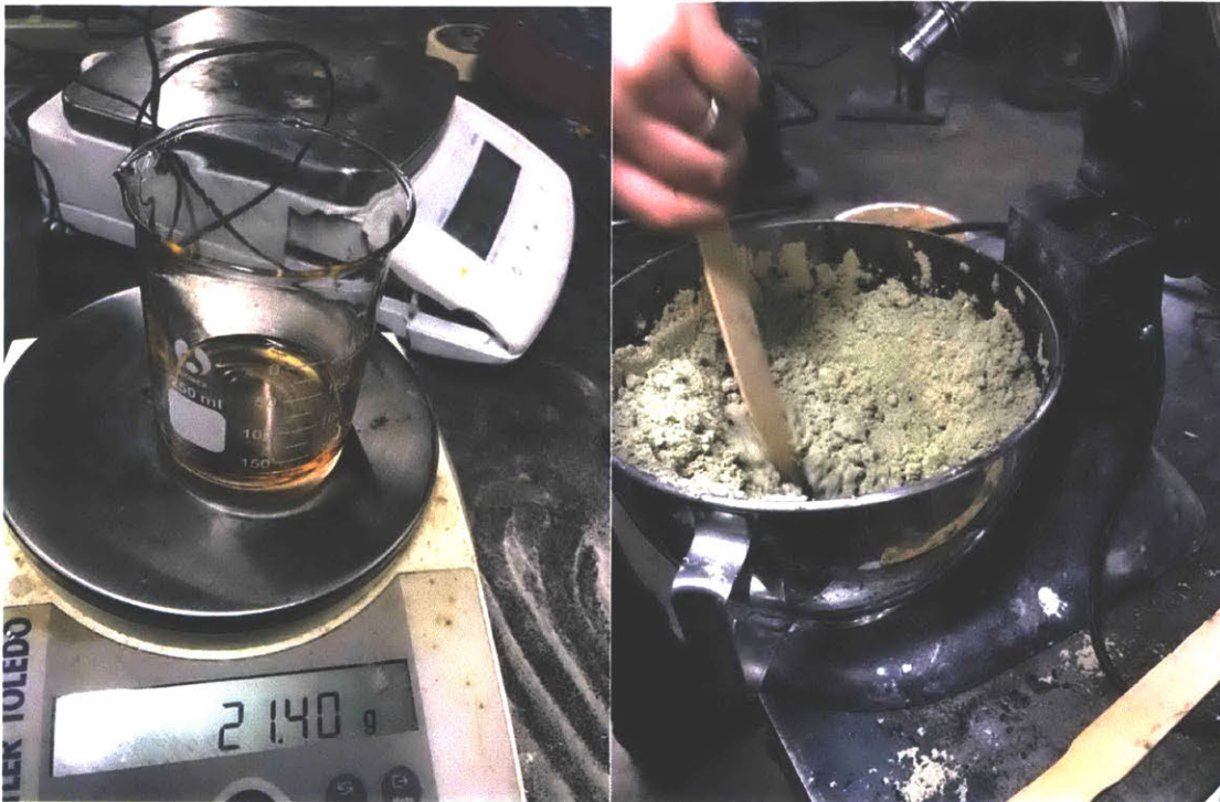
Figures 28 & 29: Catalyst is added and mixed
