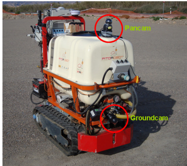
Figure 2. Position of the cameras on the tracked mobile robot used as a testbed in this research.
