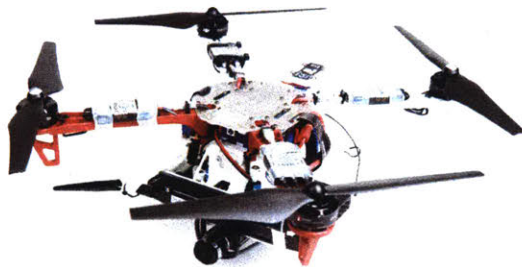
Figure 1-2: The latest iteration of the Draper-MIT autonomous quadrotor platform developed for the DARPA FLA program.
