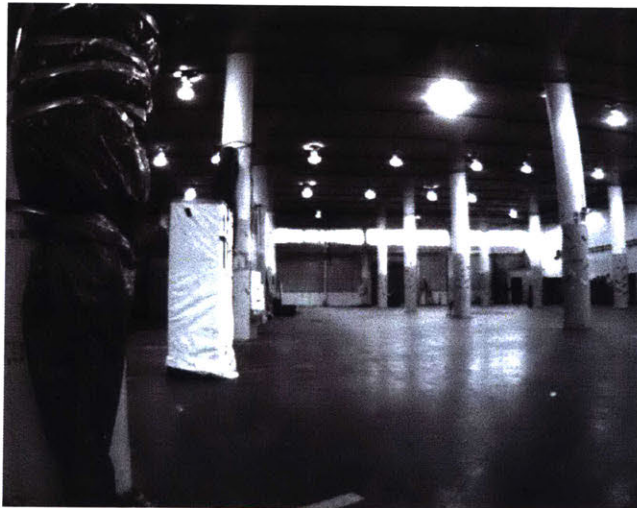
Figure 4-8: Sample image taken from the vehicle’s forward-mounted camera at the Draper-MIT warehouse test site. Note that the camera is monochrome, as is the input image to SAMWISE.
