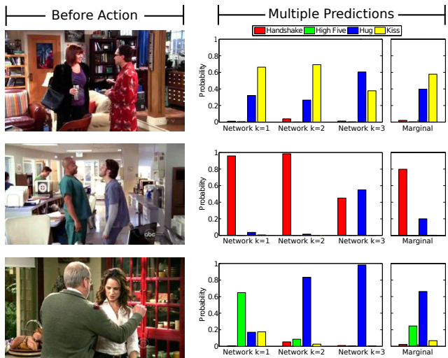
Figure 7: Multiple Predictions: Given an input frame (left), our model predicts multiple representations in the future that can each be classified into actions (middle). When the future is uncertain, each network can predict a different representation, allowing for multiple action forecasts. To obtain the most likely future action, we can marginalize the distributions from each network (right).
