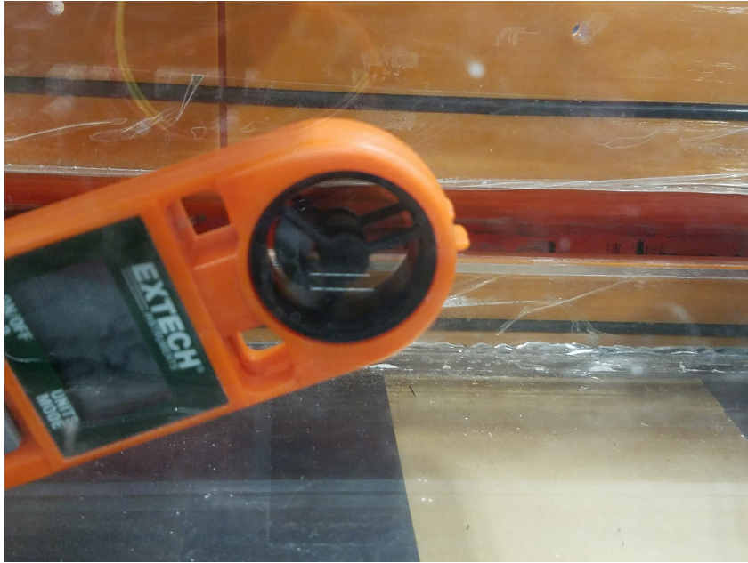
FIGURE 9: SETUP FOR VELOCITY MEASUREMENTS OF AIR EXITING THE HEAD DUCT
