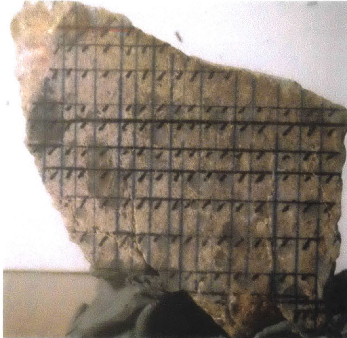
Figure 2-3: New Grid System on Flat Side. Lines were drawn on the flat side of EHJH5 after the side's strike and dip were measured. Acrylic was glued on the side shown to help prevent crumbling when the sample was cut.
