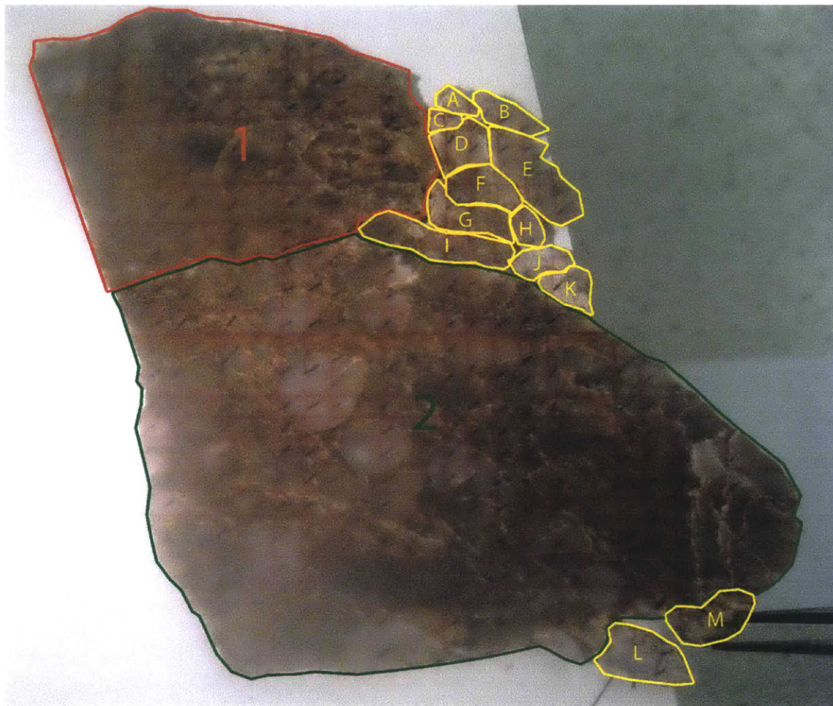
Figure 2-8: Charmander Sections. Charmander was broken into two sections in addition to pieces which crumbled off during the slab cutting. The crumbled off pieces are shown in yellow and are designated as section Charmander 0 .
