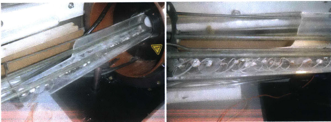
Figure 2-18: Loading Samples in Oven. (Left) To load the samples into the oven, the samples were placed in a glass "boat" which was then slid into the oven. (Right) The samples were loaded unidirectionally. For each temperature step, they were turned to face the alternating direction in/out of the oven.
