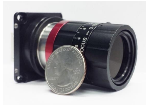
Figure 2 Laser beacon camera prototype
