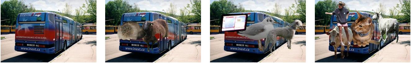
Figure 3. Examples of images in VehicleSemanticPart dataset and VehicleOcclusion dataset. The first is the original occlusion-free image from VehicleSemanticPart dataset. The second, third and fourth image (in row-major order) are from VehicleOcclusion dataset. There are 2, 3 and 4 occluders, and the occluded ratio of object, computed by pixels, is 0.2–0.4, 0.4–0.6 and 0.6–0.8, respectively.
