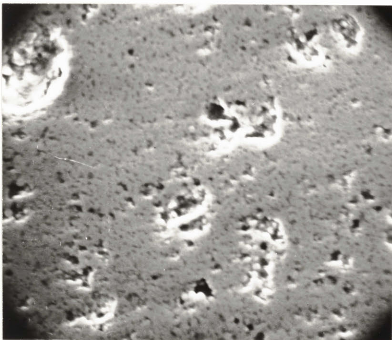
Figure III 13 ThO 2 -15 m/o ZrO 2 sintered at 1600°C, 1/2 hr., in dried high purity H 2 . Dense surface, A and porous interior B. Porosity in interior from agglomerates uncrushed by room temperature isostatic pressing. Sample HS-85-A6.
