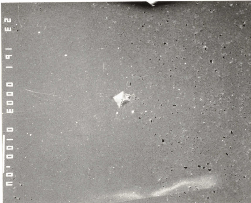
Figure III 9 Non-uniform ZrO_2 grain size distribution. Milled oxide powder dried from methanol. Annealed 10 hours, 1600^{\circ}C , CO atmosphere, sample H-85-Th 40.
