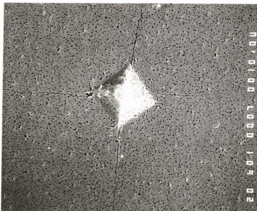
Figure IV 11 Narrow ZrO 2 grain size distribution in ThO 2 -15 m/o ZrO 2 , sample H-85-Th 40. K_{IC} = 1.5 \text{ MPam}^{1/2} @ 1 Kg.
