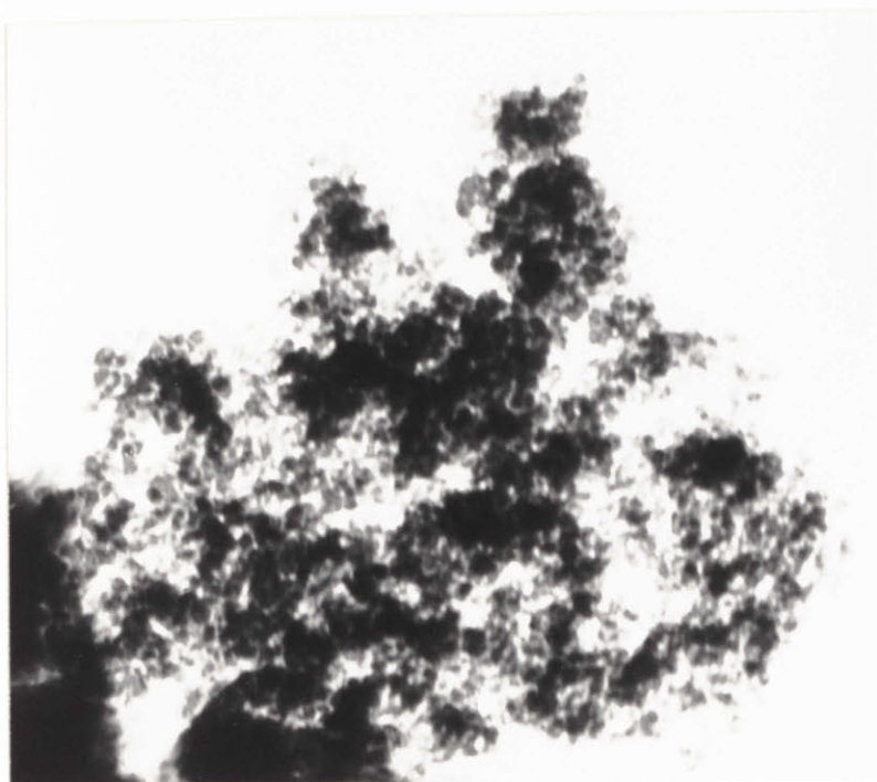
Figure III 5 Particle size of powder made from hydroxide gel. TEM picture by J. Schneibel.
