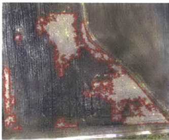
This image is a picture of weed coverage quantified using an Agrobotix UAV with collected color and infrared images after image processing. The field has roughly 16% of its surface covered by weeds.
