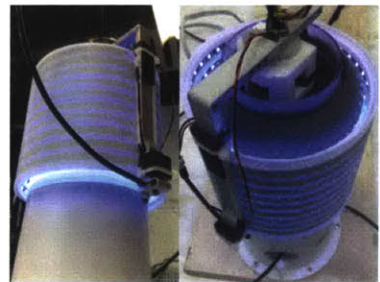
Figure 7.14: External UV LED curing cylinder, later upgraded to internal solution.
