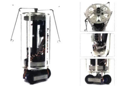
Figure 7.7: Second Fiberbot version with three wheel servo drive and linear and rotary servo control. Instead of the inflatable expandable mandrel design introduced in later versions, this robot uses a mechanical expandable design.
