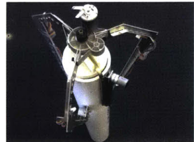
Figure 7.6: First prototype of the Fiberbot, external drive mechanism.
