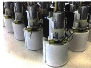
Figure 7.37: Robot inner architecture. linear stepper motor, DC air pump, solenoid valves, DC cooling fan.
