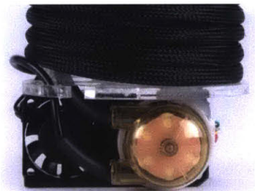
Figure 7.49: Detail of resin pump, tube wire assembly, PCB fan.
