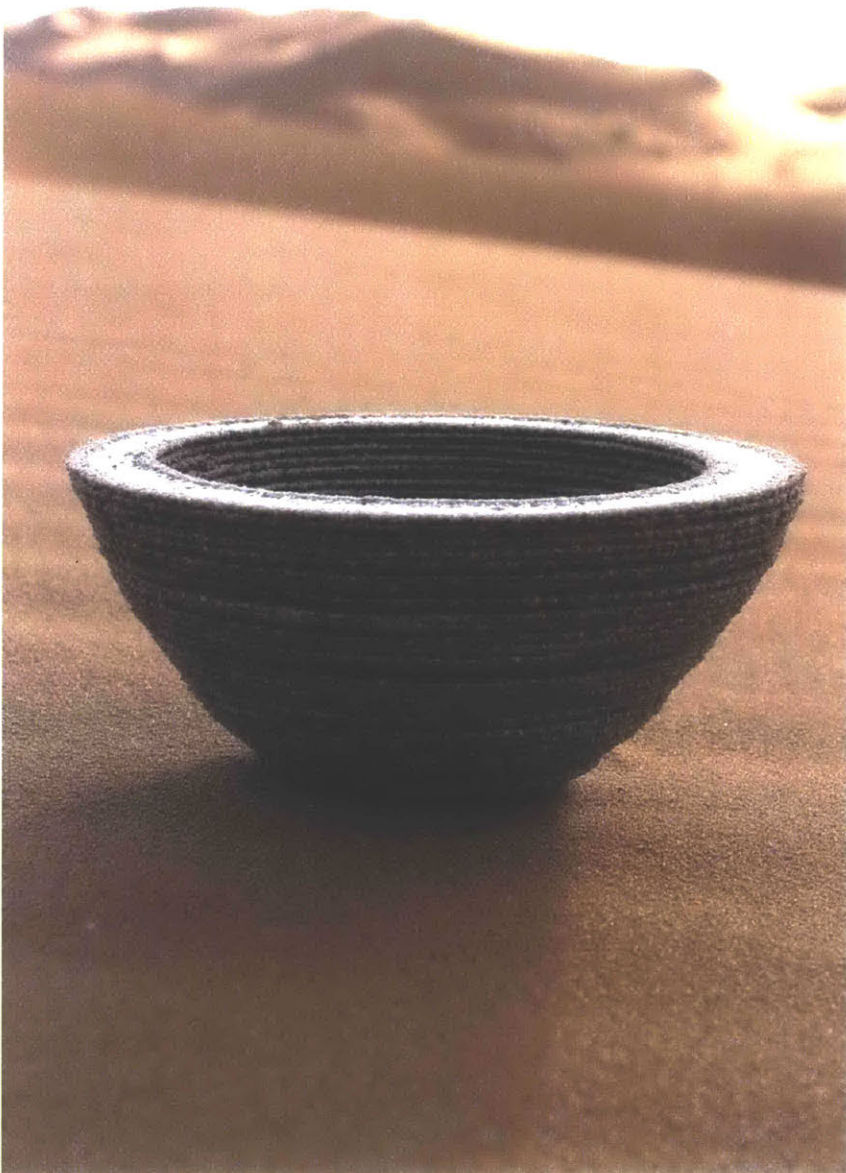
Figure 2.32: Solar-sintered bowl in the Moroccan desert. Image by the author.
