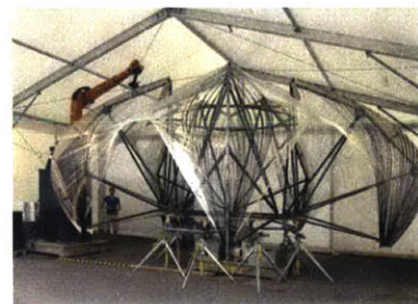
Figure 2.5: View of robotic winding process. Image reprinted from: (Reichert et al. 2014).
