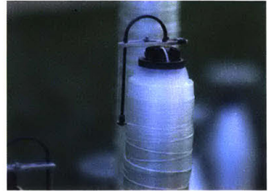
Figure 7.53: Fiberbot winding fiber, constructing a tubular member while deflating its silicone membrane.
