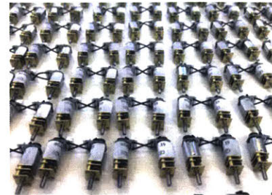
Figure 7.56: DC encoder gear motors being wired.
