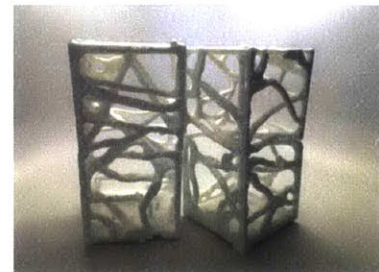
Figure 6.35: Stacks of four casts of synthetic ant environment after robotic guiding procedure.
