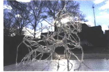
Figure 4.15: Construct printed with the multi strand extrusion approach. 40cm x 30cm in size.
