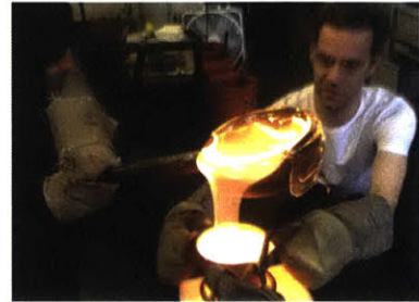
Figure 4.27: First experiments with glass extrusion at the MIT Glass Lab. Pouring glass into a crucible with an opening at the bottom. Image John Klein, Mediated Matter.
