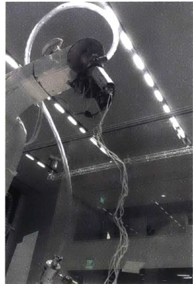
Figure 4.10: Multistrand extrusion upwards in free-space. Previously published in (Oxman, Laucks, Kayser, et al. 2013)
