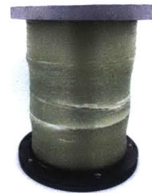
Figure 7.75: Glass fiber composite tube in aluminum fixture prepared for Instron testing by Sara Falcone, Mediated Matter.
