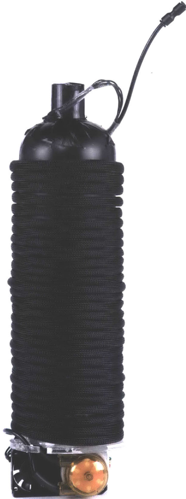
Figure 7.82: Fiberbot backend system, pump and resin bottle wrapped in wiring and tubing.
