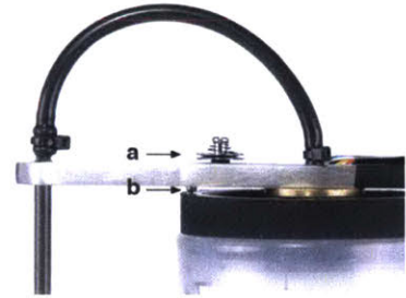
Figure 7.30: Winding arm, a.) fiber tensioner, b.) ball-nose spring plunger making contact with limit switch PCB.
