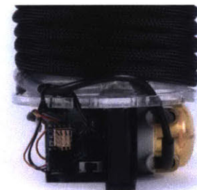
Figure 7.50: Power IN at the base supplying the robot through 7-10 m cable.
