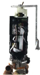
Figure 7.15: Development of the third iteration. All electronics are tightly packed inside the robot's body.
