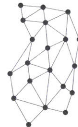
Figure 2.28: Diagram of distributed computational approach. Information is shared locally with each agent holdign equal responsibilities.
