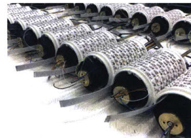
Figure 7.58: Assembly of robot inner body and rotary drive assembly.
