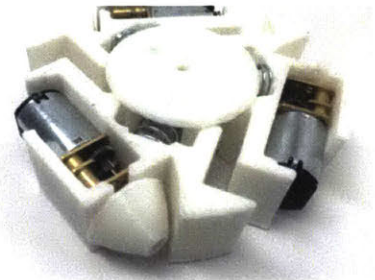
Figure 7.9: Early 3D-printed and spring-loaded base drive assembly using geared brushed DC motors.
