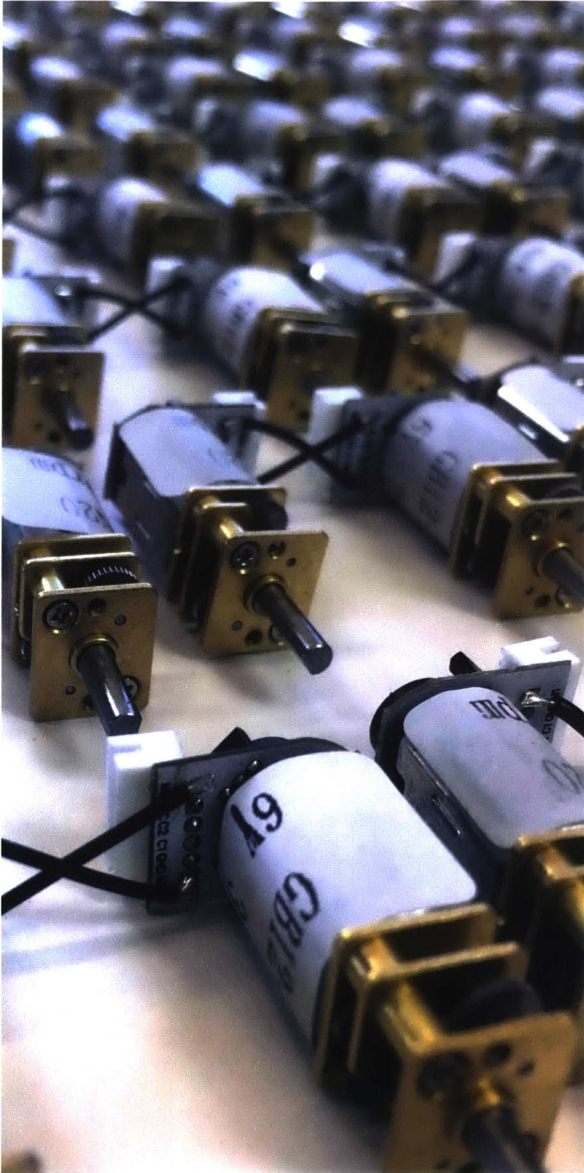
Figure 7.79: DC encoder gear motors wiring before assembly.
