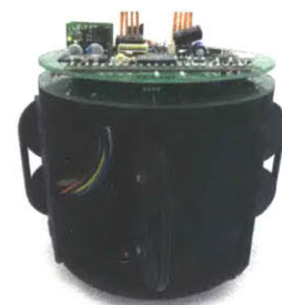
Figure 7.41: The two PCBs are stacked underneath the base drive.
