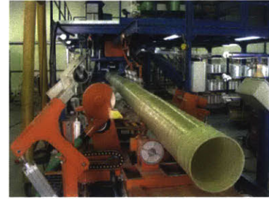
Figure 7.4: Industrial glass fiber composite filament winding machine, 'LAM-TECH Mandrel-Lamellar Machine Continuous Winder' by VEM Technologies. Image: (VEM-Technologies 2017)
