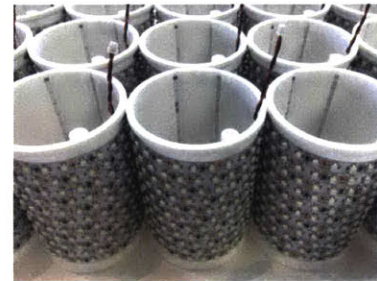
Figure 7.36: UV-curing LED assembly.
