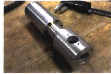
Figure 4.8: Extruder body, fabricated on the lathe from aluminum stock.
