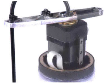
Figure 7.24: Detail of robot rotary drive assembly, winding arm, linear rail and limit switches.
