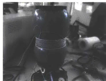
Figure 7.76: Varying the diameter of the fabricated tube by winding and inflation sequence.
