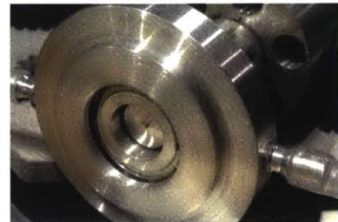
Figure 4.12: Active 360 air cooling of the nozzle area.
