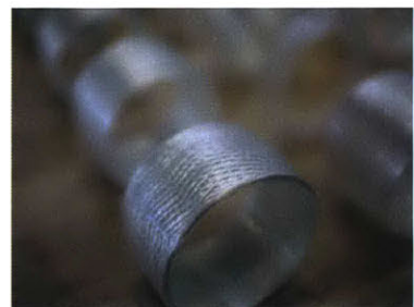
Figure 7.22: Sample with tight overlapping weave pattern and decrease resin saturation for the last layer, image Nassia Inglessis.
