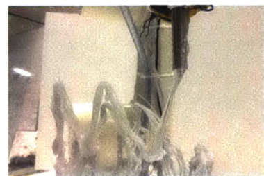
Figure 4.14: Extrusion testing re-attachment to previously cooled areas repeatedly in order to create larger constructs.
