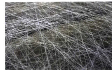
Figure 6.4: CNC deposited silk thread template.
