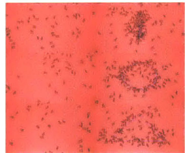
Figure 6.30: Ants accumulating around UV scanning laser in specific shapes (line, circle, triangle).
