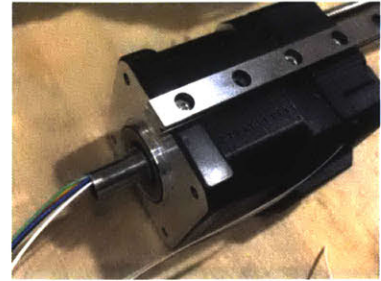
Figure 7.27: Single linear rail directly fastened to the stepper motor.
