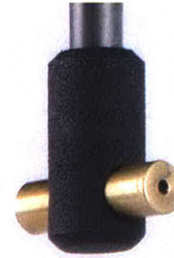
Figure 7.34: Final nozzle design. The fiber is wetted inside the nozzle right before application to the mandrel.
