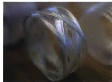
Figure 7.21: Layered cross-wind with matching overlap, creating a lattice. Image: Nassia Inglessis.
