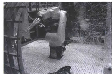
Figure 4.18: Fiber pulling tool on robotic arm, wooden scaffold structure with hooks. Previously published in (Oxman, Kayser, et al. 2013)
