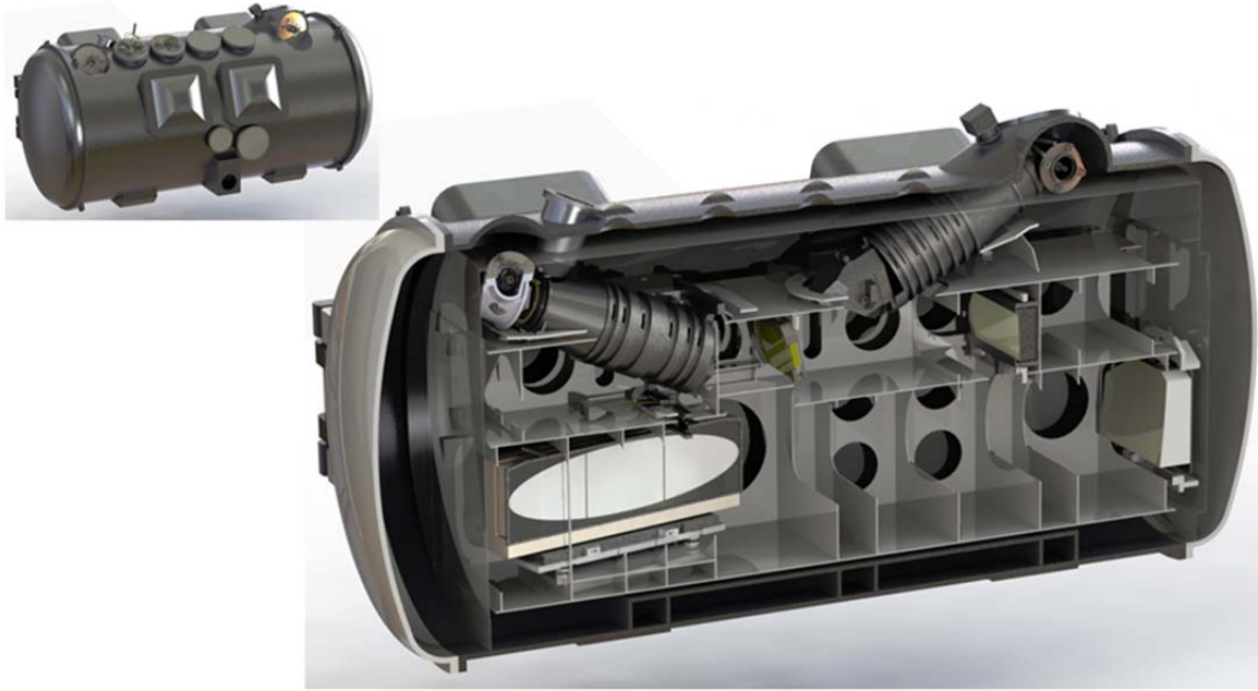
Figure 9 – Cylindrical Vacuum Chamber Concept with Section View
