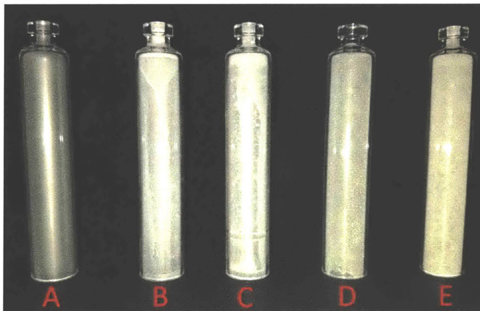
Figure 34: Powder Coated Samples. A: Unsiliconized sample with powder coating; B: Flushing sample unbaked; C: Flushing sample baked (note line where stopper was placed); D: Microdosing sample unbaked; E: Microdosing sample baked
