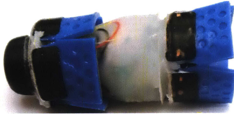
Figure 5-25: Robot prototype with the tactile speed sensor for measuring instantaneous speed at every in-pipe obstruction
