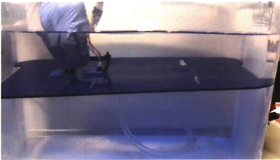
Figure 4-22: Actual experiment setup for testing the new leak sensors' ability to tell leaks and obstructions apart
