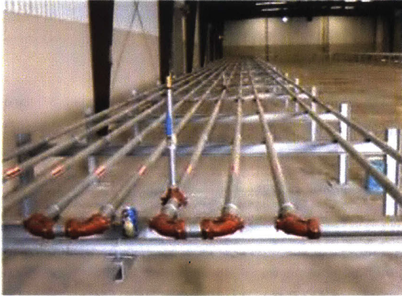
Figure 2-1: A 1.5km long, 52mm inner diameter, cast iron pipe loop for testing pipeline technologies in industrial settings.
