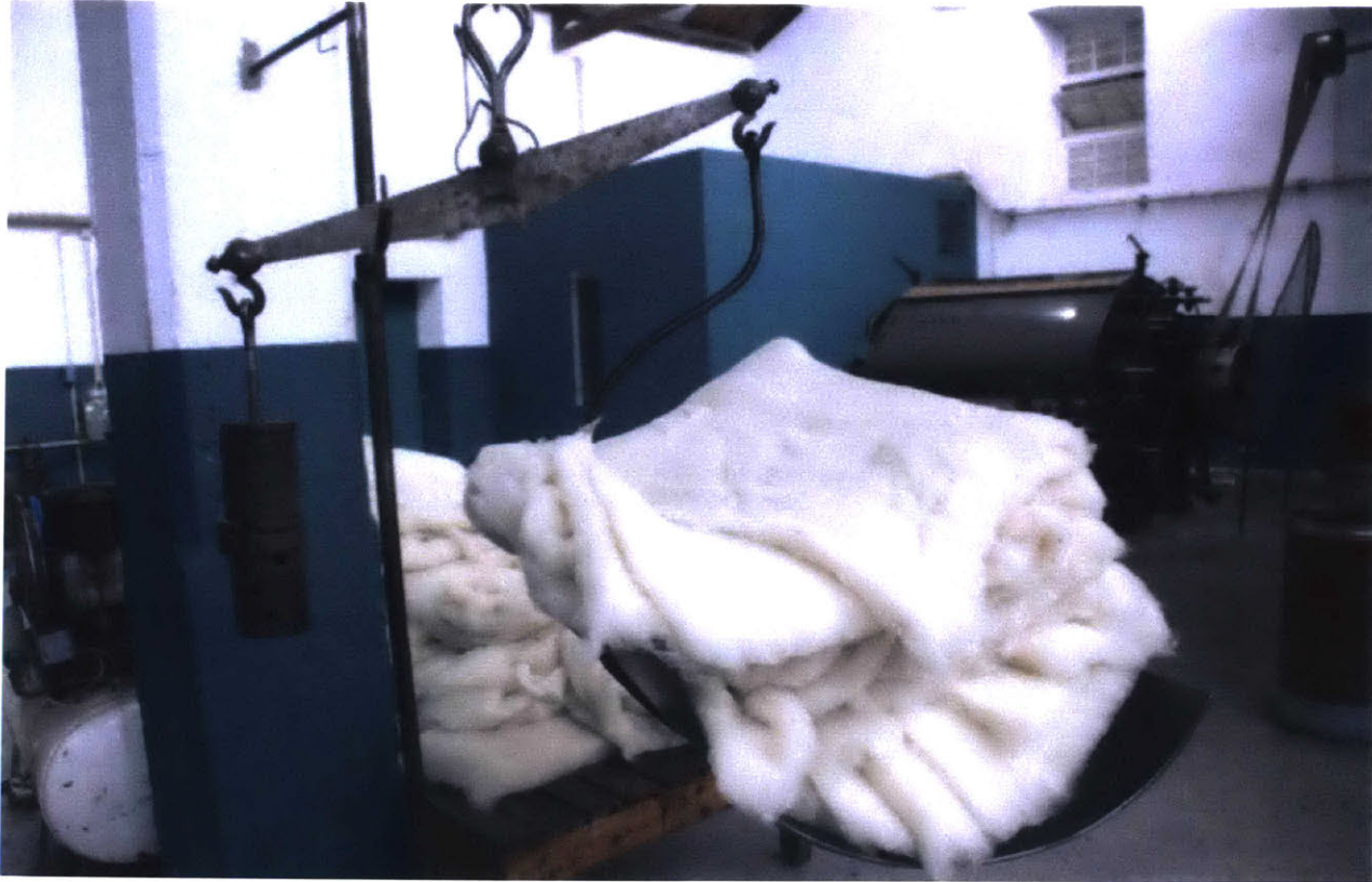
The sliver is weighed before being drawn and amalgamated onto roving rolls.
