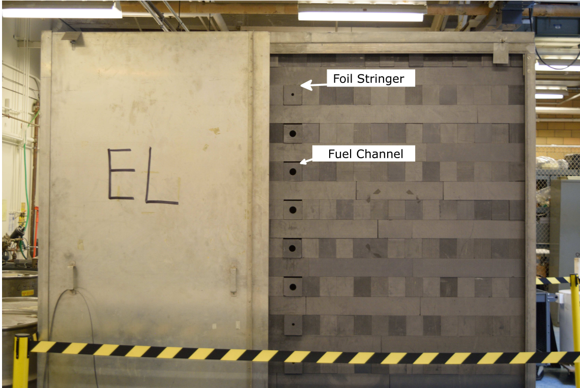
Figure 2.2: The Graphite Exponential Pile East face. Only one cover is removed from this face. Here both types of neutron measuring blocks can be seen. These blocks are removable and can be moved to create a desired configuration. The extra fuel channels have been re-purposed for use with neutron detector probes.
