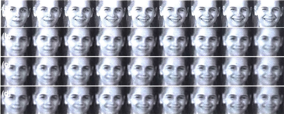
Figure 2-5: Results from reconstruction using multi velocity encoders, bottom 3 images are output from autoencoder ensemble. (a) Input video sequence from MMI dataset ([72]). (b) Reconstruction using encoder with sampling factor of 1/3 . (c) Reconstruction using sampling factor of 2/3 . (d) Reconstruction at original velocity.
