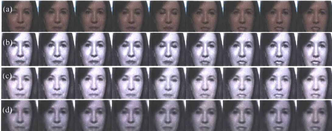
Figure 2-4: Results from reconstruction using temporal convolutional autoencoder on a face video. (a) Input video sequence. (b) Reconstruction after using 4 convolutional layers. (c) Reconstruction after using 8 layers. (d) Reconstruction after using 12 layers.
