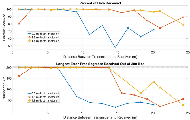
Figure A-3: Acoustic range tests: Results of transmitting a sequence of 200 alternating bits at 20 bits/s at various depths and distances, in order to characterize the acoustic communication performance.
