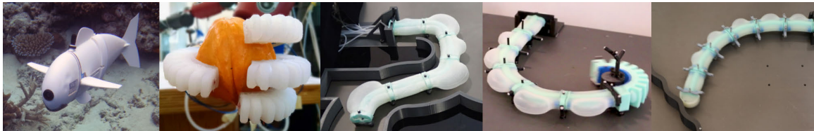
Figure 3-15: Soft robots developed in this thesis. Left to right: soft robotic fish (SoFi) (Section 3.6.1 and Chapter 4), soft gripper hand (Sections 3.6.2, 3.6.3, and 7.1.2), cylindrical multi-segment arm (Sections 3.6.6 and 7.1.1), pleated gripper on multi-segment arm (Sections 3.6.5 and 7.1.3), and soft hemisphere on multi-segment arm (Sections 3.6.8 and 7.2.2). Some of the images are adapted from Katzschmann et al. [2018b], Homberg et al. [2018], Marchese et al. [2014a], and Katzschmann et al. [2015].
