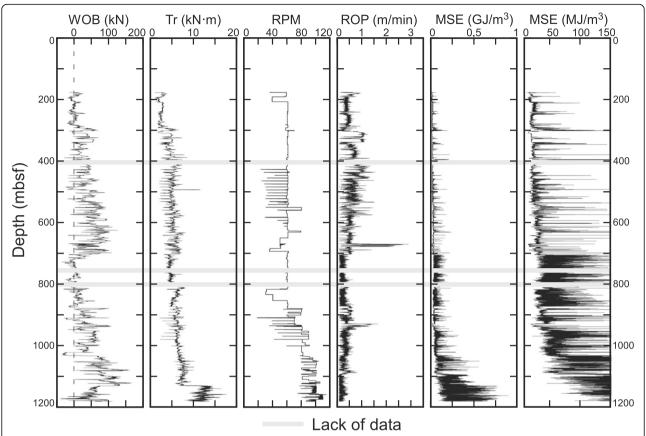
**Fig. 2** Examples of drilling performance parameters collected at site C0023. WOB, Tr, and RPM data were sampled at the surface every second. ROP was recalculated using bit depth data recorded in the same manner as that of the other drilling parameters. Abbreviations in the inset include *WOB* weight on bit, *Tr* torque, *RPM* rotations per minute, *ROP* rate of penetration, *MSE* mechanical specific energy
