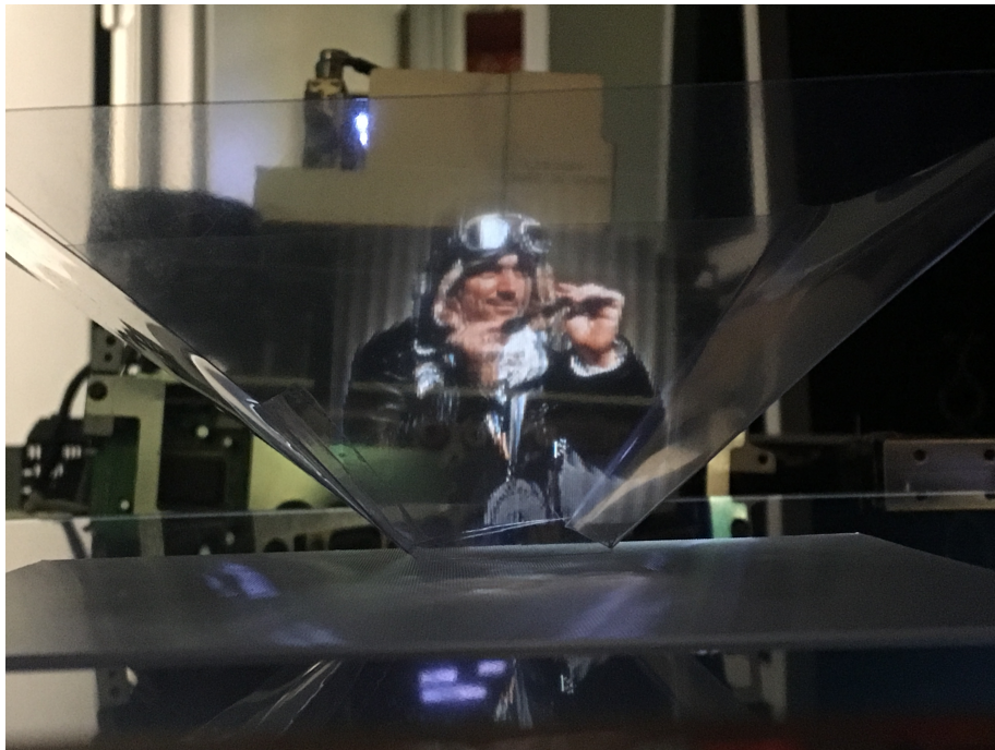
FIGURE 4.8: A promising final resulting 3-Dimensional autostereoscopic display with a combination method of Pepper's Ghost and lenticular imaging on a 4K monitor.
