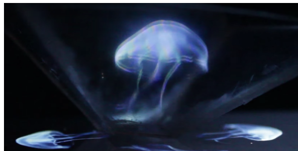
FIGURE 3.2: A simple Pepper's Ghost illusion created with an iPhone, a piece of transparency, and tape. Shaw [24].
