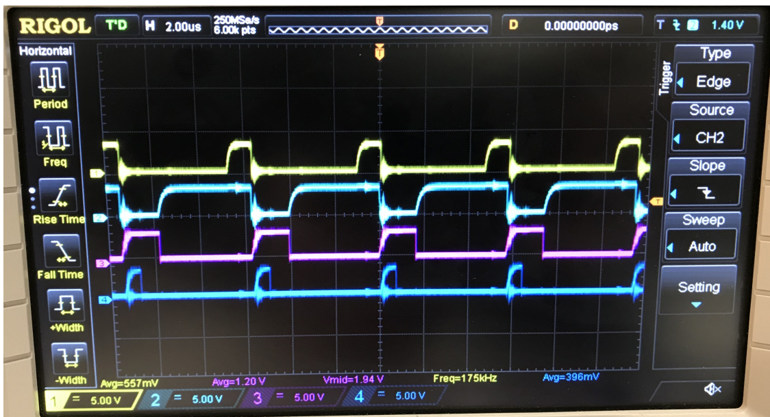
Figure 5-13: Three Level Buck control signals when V_{out} \approx V_{in}/2 . From top to bottom the signals are Q_1 , Q_2 , Q_3 , and Q_4 .
