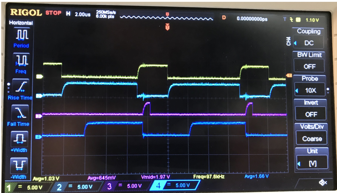
Figure 5-20: ResSC control signals when V_{out} \approx V_{in}/2 . From top to bottom the signals are Q1, Q2, Q3, and Q4.
