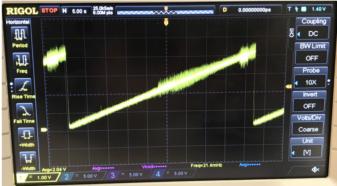
Figure 5-16: Output voltage ramp of Three Level Buck over 45s with no offset in phase from 180deg.
