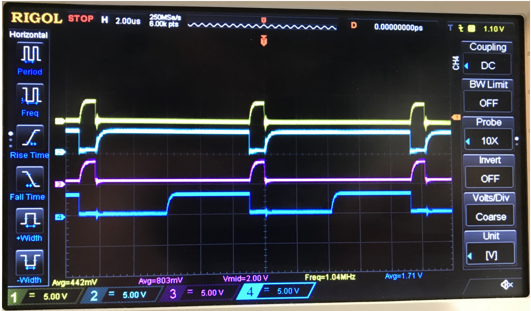
Figure 5-19: ResSC control signals when V_{out} < V_{in}/2 . From top to bottom the signals are Q1, Q2, Q3, and Q4.
