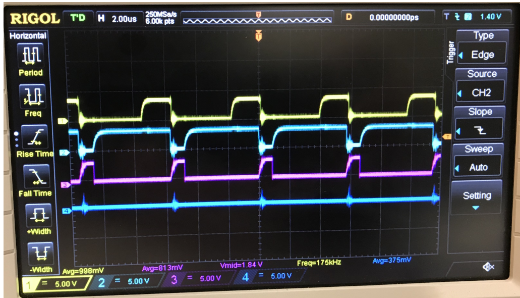
Figure 5-14: Three Level Buck control signals when V_{out} > V_{in}/2 . From top to bottom the signals are Q_1 , Q_2 , Q_3 , and Q_4 .
