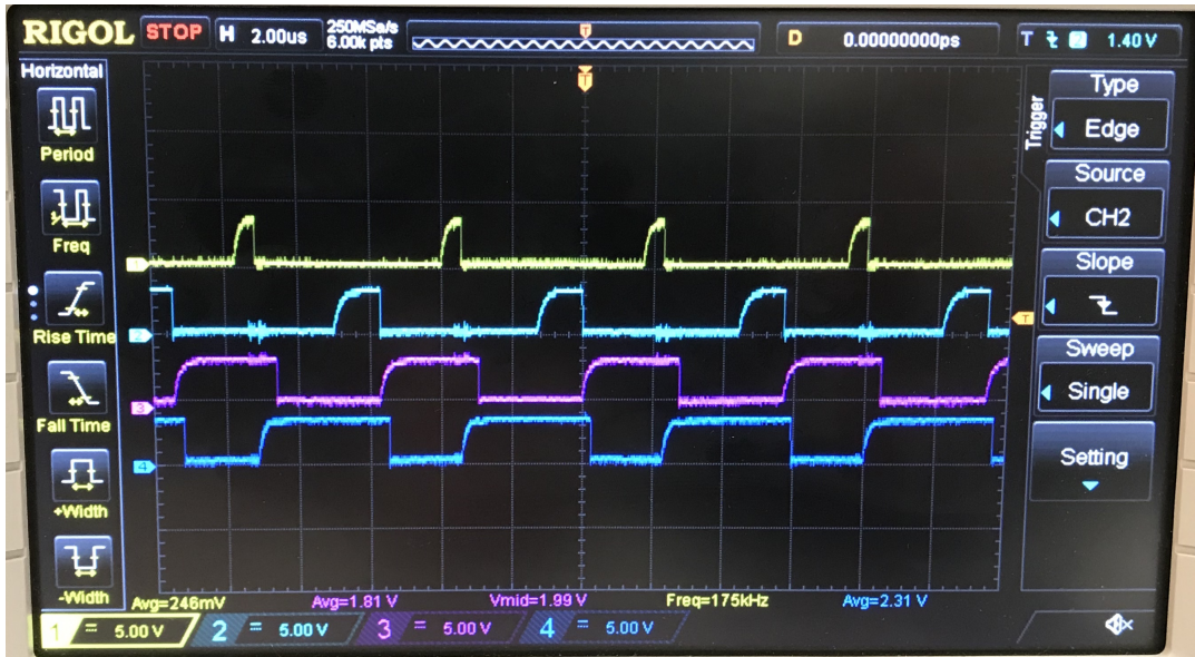
Figure 5-12: Three Level Buck control signals when V_{out} < V_{in}/2 . From top to bottom the signals are Q_1 , Q_2 , Q_3 , and Q_4 .
