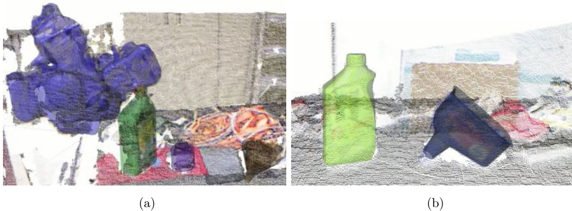
Figure 5-16: Object Pose Estimates in Real-World Experiment 2 Object pose estimates from Real-World Experiment 2 are shown as object mesh models rendered at the estimated pose. Note how closely the object meshes align with the raw point cloud.
