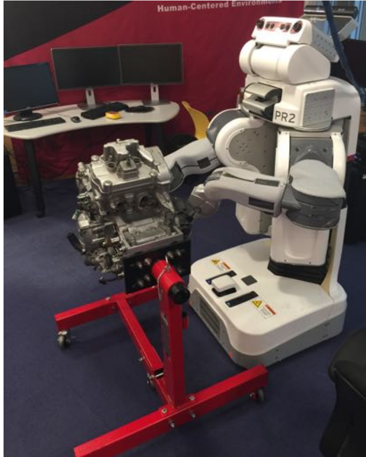
Figure 1-1: Example of a robot in a real-world environment. The robot needs to be aware of the identity and location of objects in its surroundings to robustly perform tasks such as collision-free navigation, object manipulation, and task planning.
