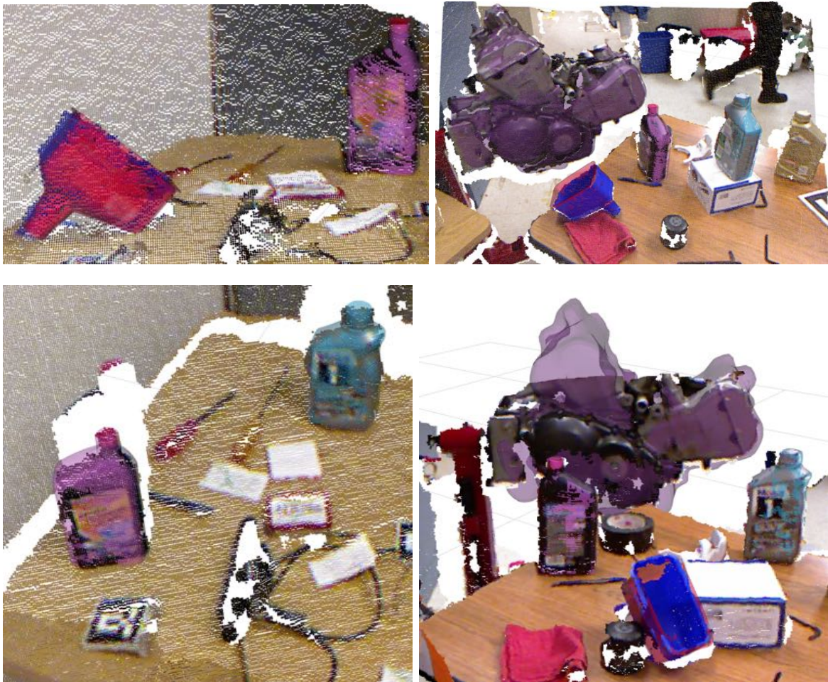
Figure 5-15: Various Object Pose Estimates in Real-World Experiment 1 Object pose estimates from various trials in Real-World Experiment 1 are shown as object mesh models rendered at their estimated poses. Note how closely the object meshes align with the scene point cloud. The blue mesh corresponds to the gray oil bottle, the red mesh corresponds to the blue funnel, the pink mesh corresponds to the black bottle, and the purple mesh corresponds to the engine.
