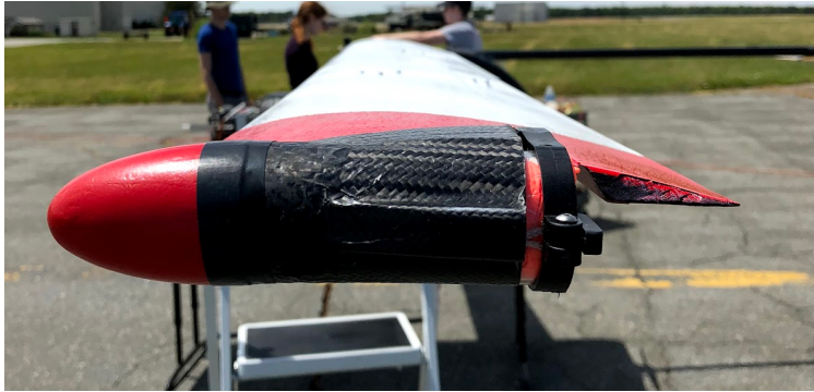
Figure 2.12: Installed flight termination system on left wing.
