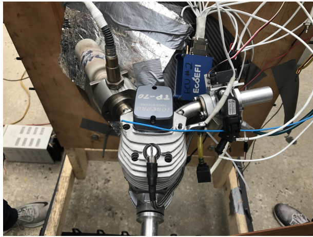
(a) TP70 ground test on stand
