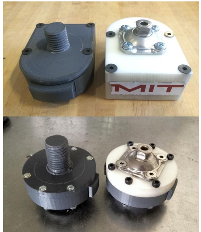
Figure 5. FULLY ASSEMBLED PROTOTYPES A AND B WITH BOTH THE PROPRIETARY SCREW CONNECTOR FROM THE JAIPURFOOT ORGANIZATION AND THE MORE UNIVERSAL PYRAMID CONNECTORS USED AT MOBILITY INDIA.
