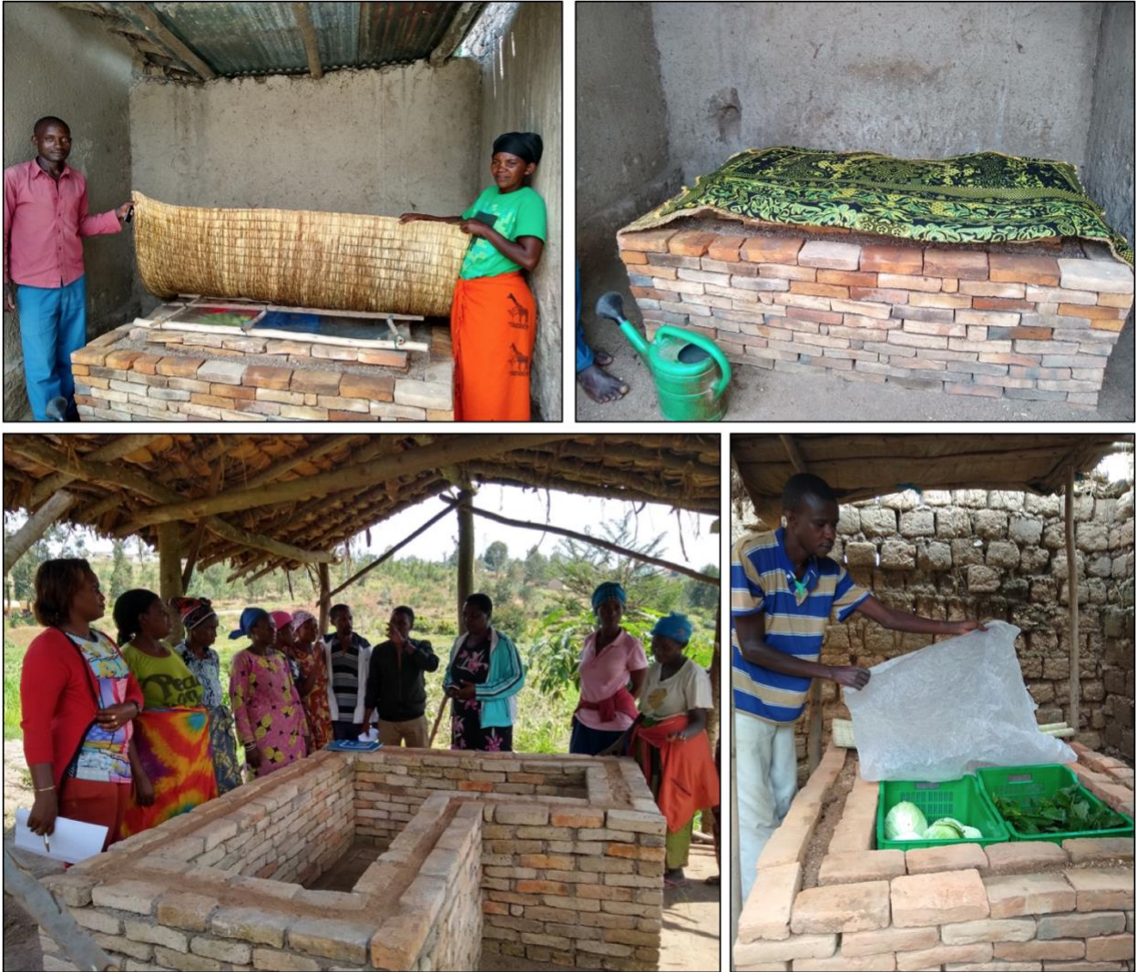
Above are images of a brick evaporative cooling device at various locations in Rwanda.
