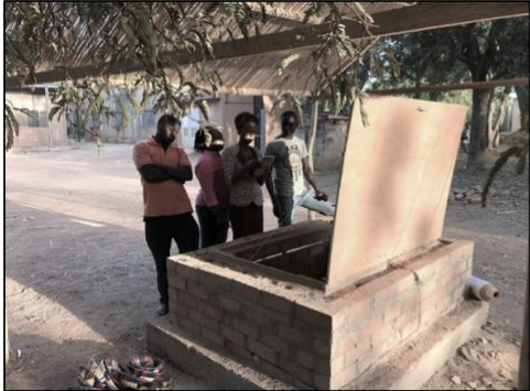
Above are images of a brick evaporative cooling device in Kamboinse, Burkina Faso.
