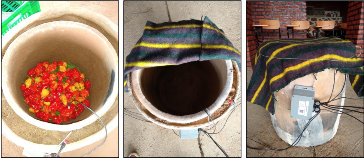
Above are images of clay pot coolers with a clay pot in clay pot configuration at various locations in Rwanda.
