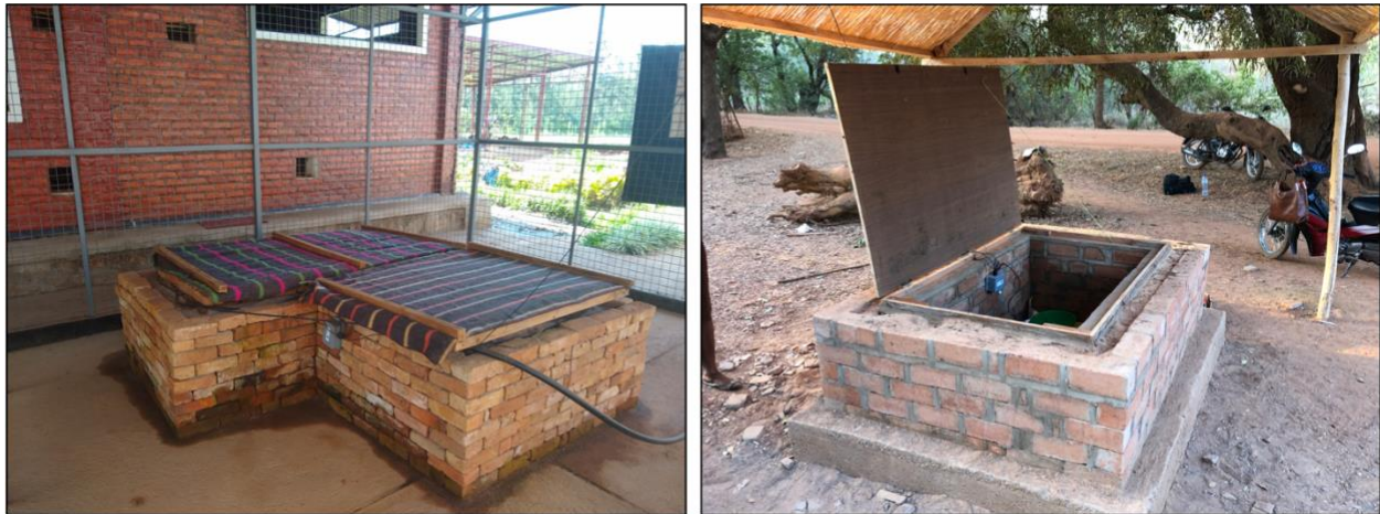
Figure 8. Left: ZECC in Mulindi, Rwanda with bricks that are stacked, a cloth cover supported by a wood and straw frame, and a structure with a tightly woven straw roof providing shade a majority of the day.
