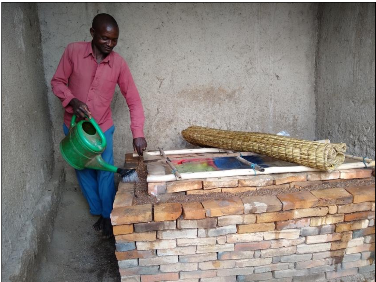
Figure 2. Brick evaporative cooling device in Rubona, Rwanda.
