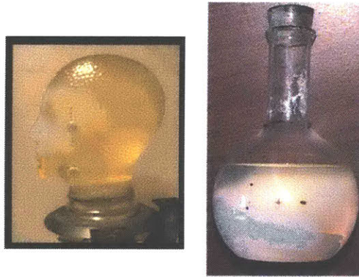
Figure 11: Two different gel dosimeters, initially transparent then irradiated. The regions of color and opacity change mark the region of irradiation [43].
