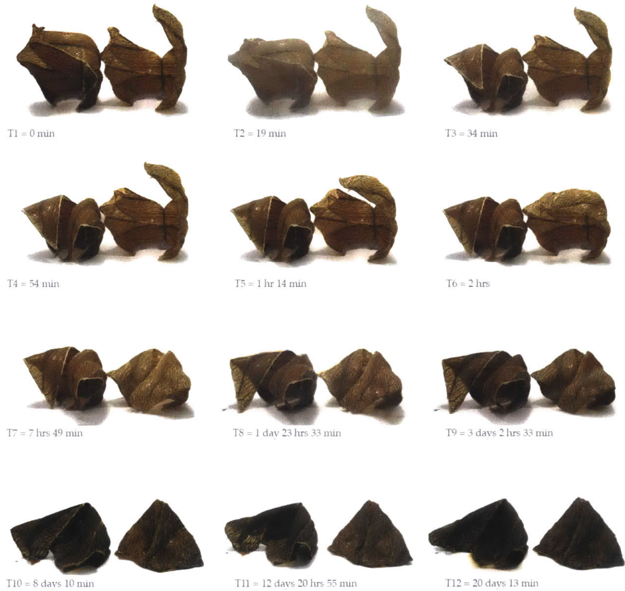
Figure 1.19 — Water-induced failure of maquettes in high ambient temperature and relative humidity, over a period of 20 days
