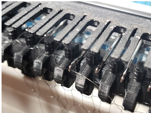
(d) The needle's latch closed
