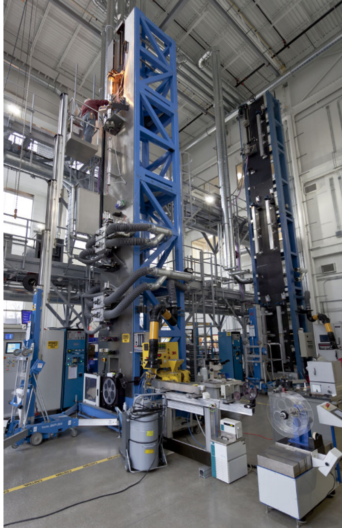
Figure 1-1: The example an industrial optical fiber draw tower [1]
