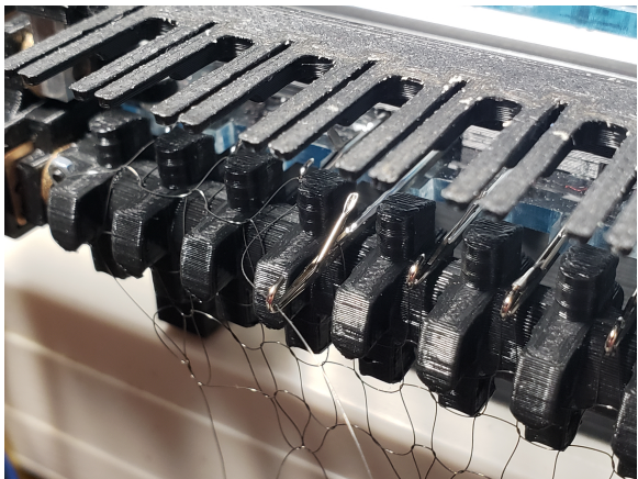
(c) Needle being retracted forming a new knit
