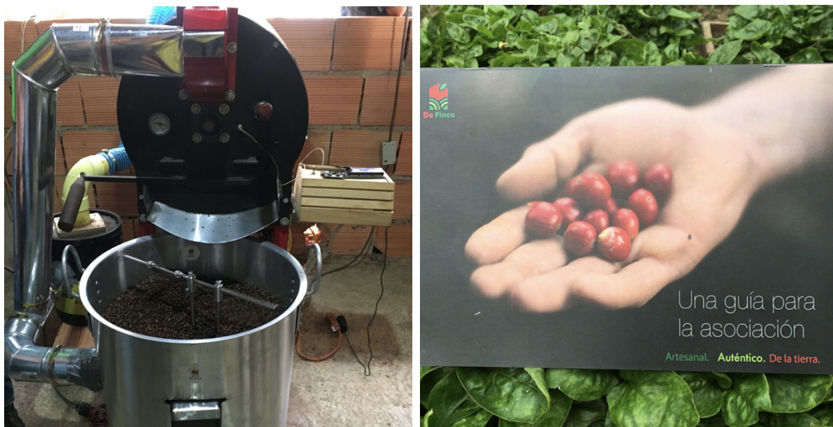
Figure 4. Selection of projects developed with the DeFinca community. Low-cost coffee roaster with smoke extraction and coffee bean cooling systems integrated (left). Guide to onboarding and management of association members (right).
