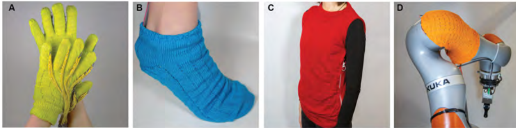
Figure 4-6: Automated manufactured full-size tactile A. glove, B. sock, C. vest and D. robot arm sleeve.
