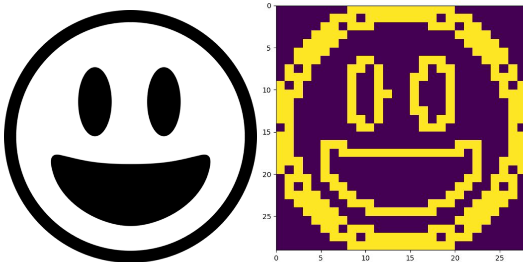
Figure 21: High resolution input image (left) and TactionTablet compatible output (right)
