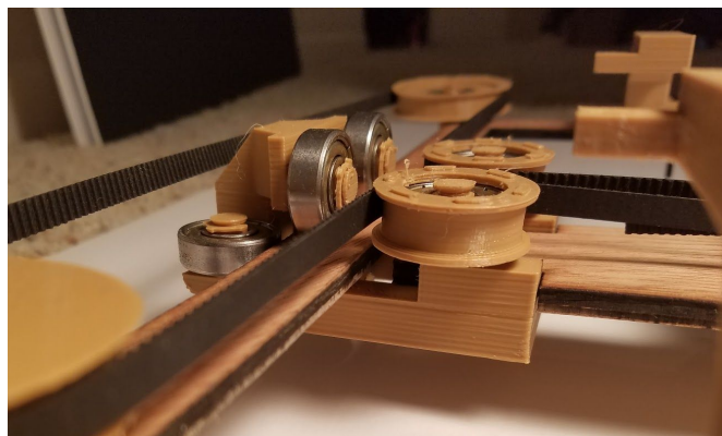
Figure 7: X-carriage size view with clips to hold on bearings
