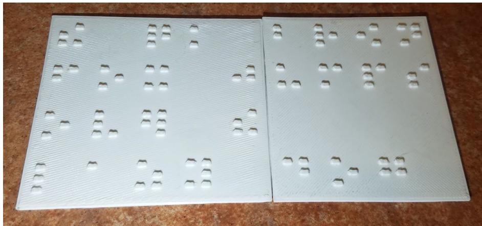
Figure 23: Braille 3D printed at the pitch of the TactionTablet
