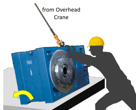
Figure 1-1: Workers must often work with cranes in order to tumble heavy objects about a contact point on the ground. This is done to gain access to otherwise obscured faces of the object.
