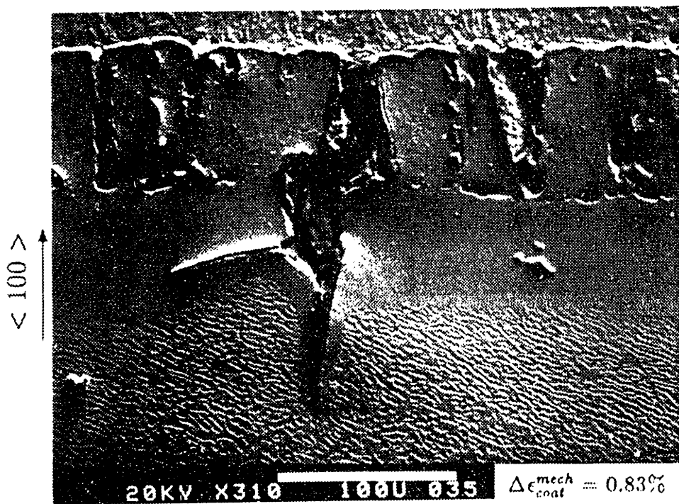
(b) After cyclic exposure (6000 4.5s heating cycle) showing grain boundary oxidation, and crack propagation into the substrate
