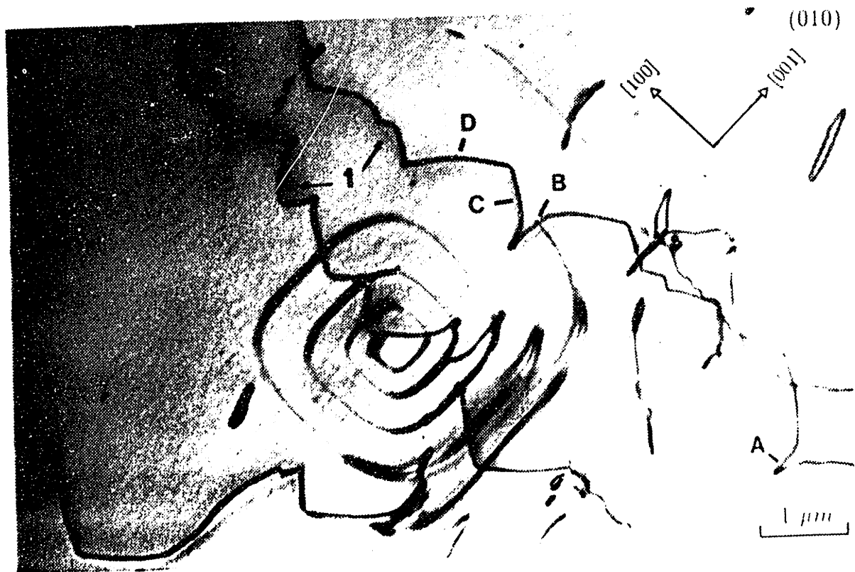
Fig. 4.6 Electron micrograph showing a helical dislocation and sharply kinked or zig-zag dislocations
