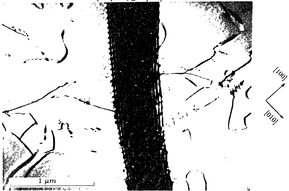
(b) Dense band of dislocations forming cell walls. (001) foil, g = [\bar{1}\bar{1}0]
