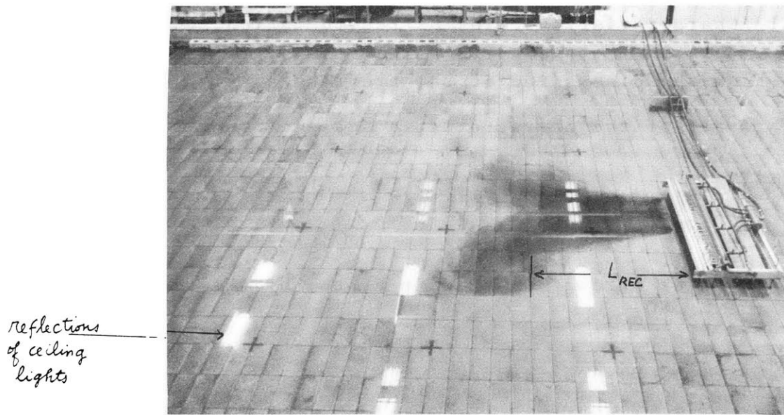
Fig. 8-2 a. Recirculation demonstrated in a full diffuser test (MJ 23) : immediately following dye injection
