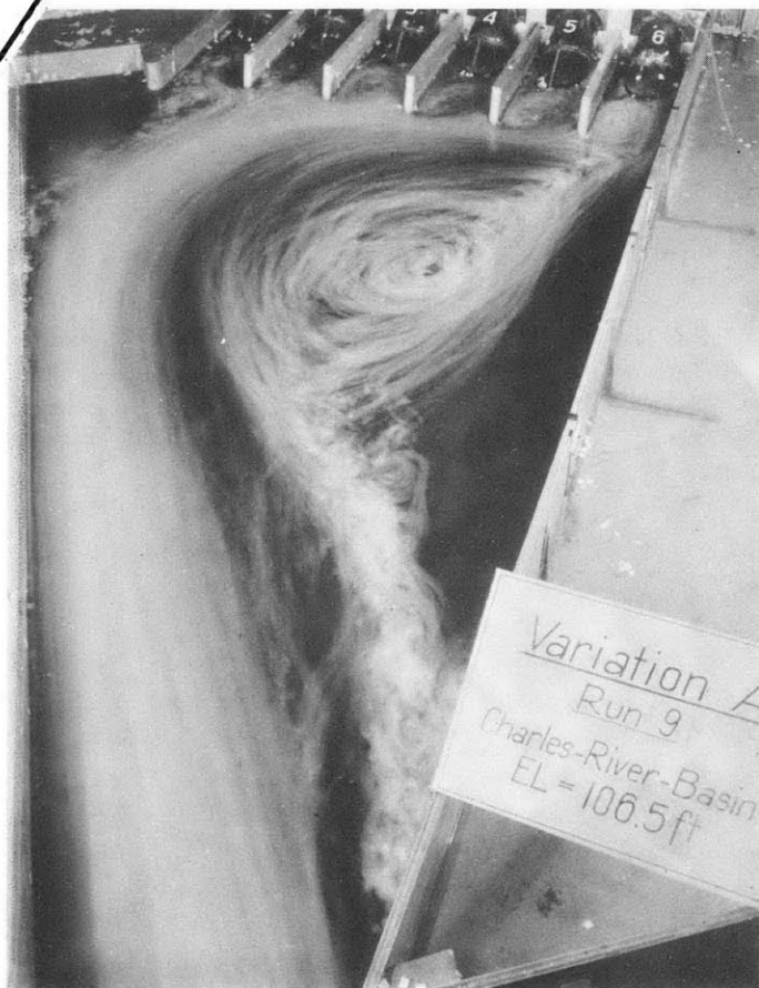
Fig. 12: Forebay Flow Pattern, Variation A. Each Intake Withdrawing 1400 cfs.
