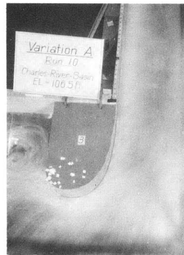
- 3 - well streamlined pier with 36 ft. base width
