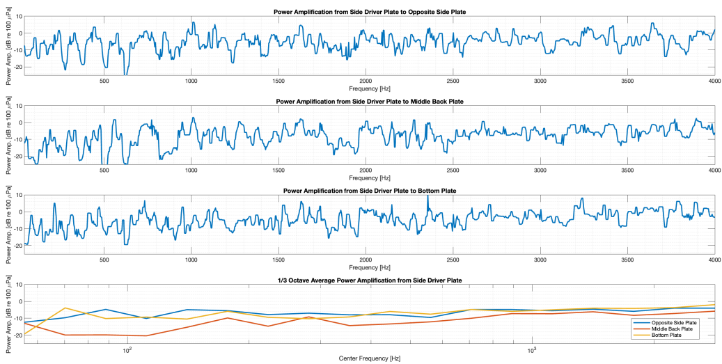
Figure 2-8: Power Amplification Values using FEA
