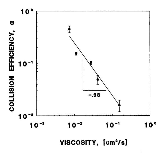
Figure 6-13. Collision efficiency of CRL 1606 cells versus viscosity using 500,000 MW dextran as viscosity enhancer at 215 mg PLH/m<sup>2</sup>, shear rate = 30 s<sup>-1</sup>.
