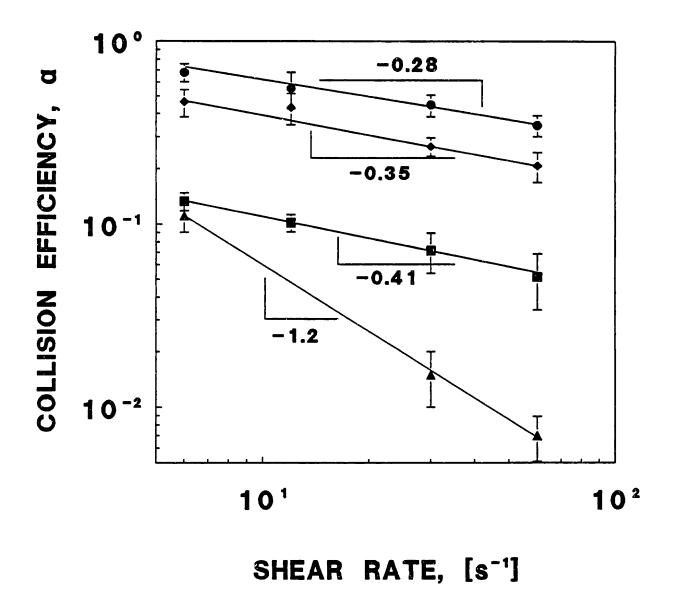
Figure 6-12. Collision efficiency of CRL 1606 cells versus shear rate at various polymer doses. ▲ - 12 mg/m², ■ - 40 mg/m², ♦ - 133 mg/m², ● - 215 mg/m².
