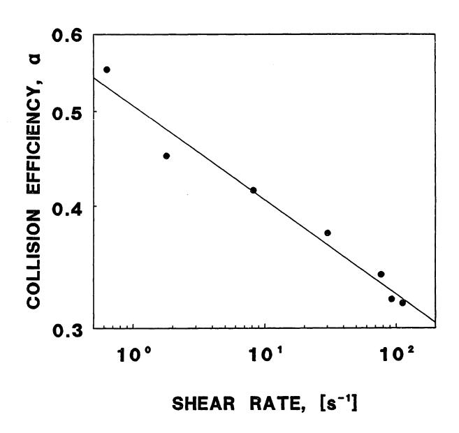
Figure 3-6. Collision efficiency of salt coagulated latex versus fluid shear rate from the data of Curtis and Hocking (1970).
