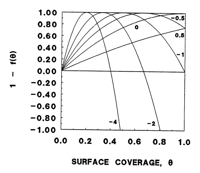
Figure 6-2. [1- $f(\theta)$ ] versus fractional surface coverage for w = 1 and various  $z_p$ .  $z_p$  values are indicated on the figure.
