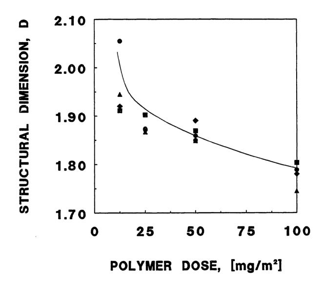
Figure 7-4. Fractal dimension for CRL 1606 flocs versus polymer dose at various shear rates.  $\bullet$  - 53 s<sup>-1</sup>,  $\blacktriangle$  - 32 s<sup>-1</sup>,  $\bullet$  - 12 s<sup>-1</sup>,  $\blacksquare$  - 5.3 s<sup>-1</sup>.
