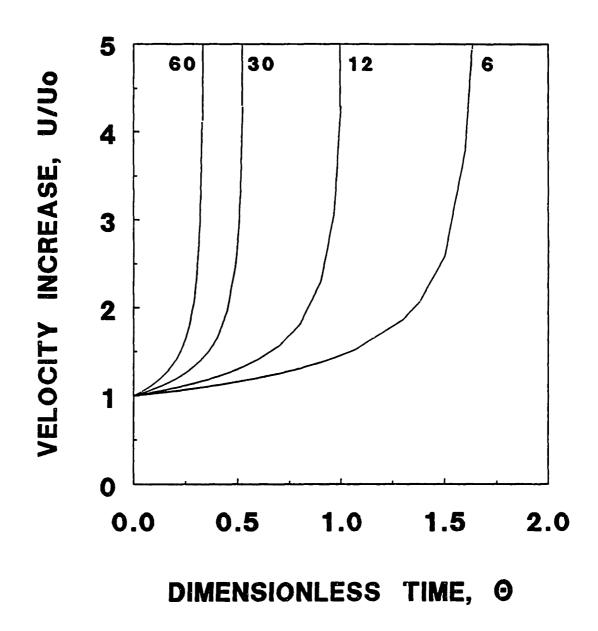
Figure 8-6. Sedimentary velocity enhancement versus dimensionless time predicted by equations (8-10), (8-15) and (8-16) for a polymer dose of 40 mg PLH/m<sup>2</sup>, using the experimental data from chapters 6 and 7. The values of fluid shear rate are shown on the figure.
