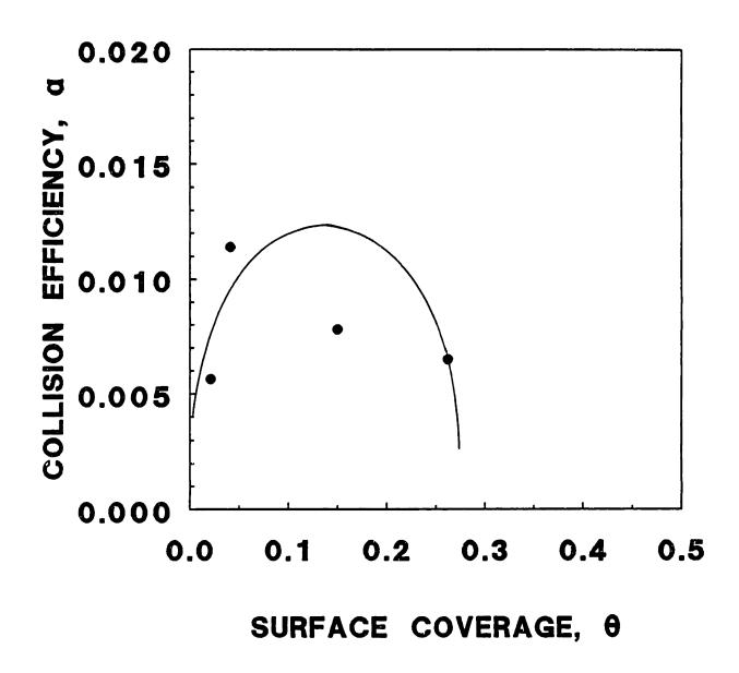
Figure 3-4. Collision efficiency of alum flocculated silica versus calculated fractional surface coverage from the data of Hahn and Stumm (1968).
