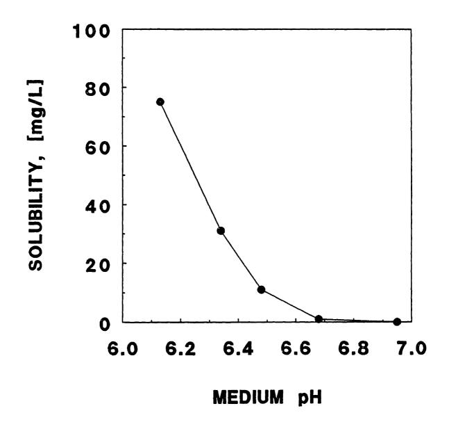
Figure 5-4. Solubility of poly-L-histidine, 23,000 MW, in 0.15 M NaCl versus pH.
