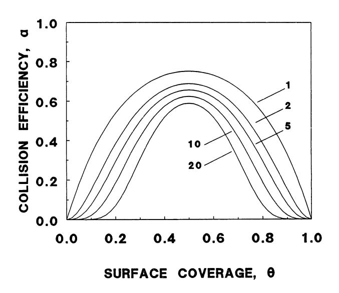
Figure 6-3. Collision efficiency versus fractional surface coverage predicted by equations (6-7) and (6-9) for various n, and m = n/2.
