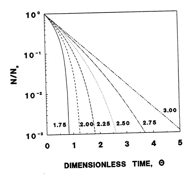
Figure 8-1. Normalized particle concentration versus dimensionless time for various fractal dimensions, with  $\alpha = 1$ ,  $\dot{\gamma} = 1$  s<sup>-1</sup>.
