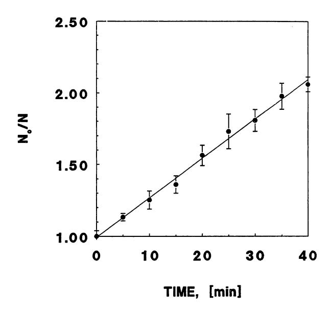
Figure 4-1. Inverse normal particle concentration,  $N_o/N$ , versus time for a typical collision efficiency experiment.  $N_o = 50,100$  cells/mL,  $a = 7.8 \mu m$ , 26 mg PLH/m<sup>2</sup>, shear rate = 12 s<sup>-1</sup>.
