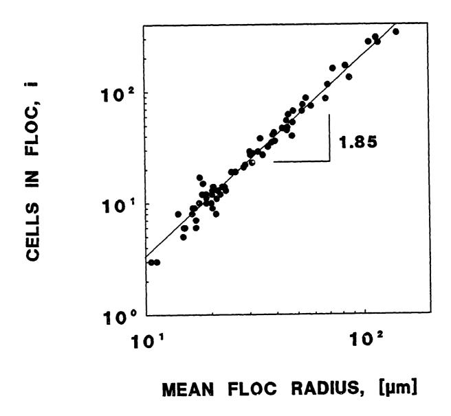
Figure 7-3. Number of cells in CRL 1606 flocs versus the geometric mean radius of the floc, for 50 mg/m<sup>2</sup> poly-L-histidine flocculant dose and 30 s<sup>-1</sup> shear rate.
