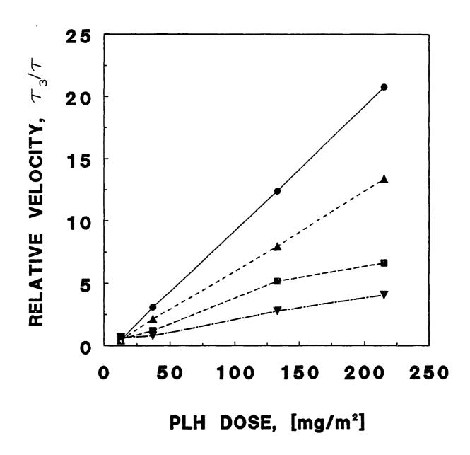
Figure 8-2. Experimental normalized flocculation rate constants versus poly-L-histidine dose at various shear rates. ▼ - 6 s<sup>-1</sup>, ■ - 12 s<sup>-1</sup>, ▲ 30 s<sup>-1</sup>, ● - 60 s<sup>-1</sup>.
