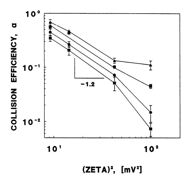
Figure 6-6. Experimental collision efficiency of CRL 1606 cells versus zeta potential squared at various shear rates. ■ - 6 s<sup>-1</sup>, ◆ - 12 s<sup>-1</sup>, ◆ - 30 s<sup>-1</sup>, ▲ - 60 s<sup>-1</sup>.
