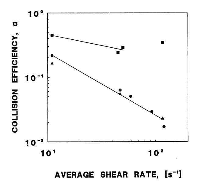
Figure 3-5. Collision efficiency of polyethylenimine flocculated latex versus fluid shear rate from the data of Birkner and Morgan (1968).
