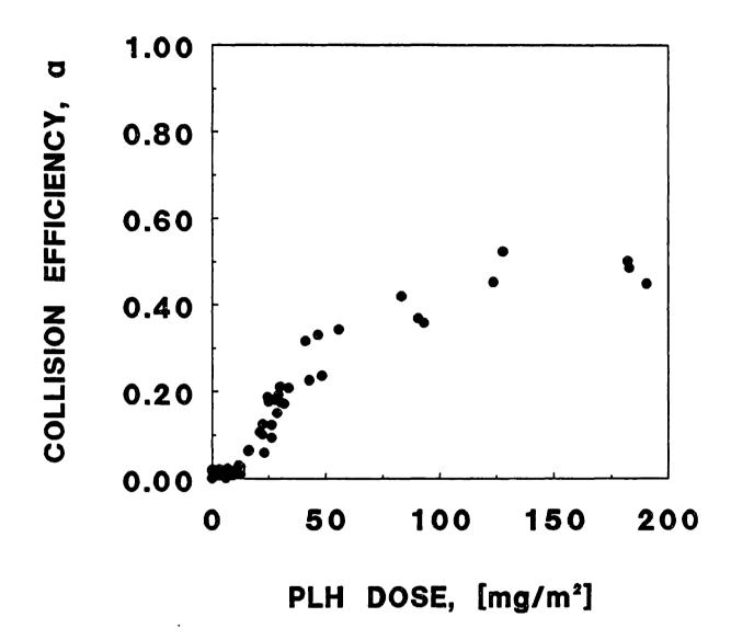
Figure 6-7. Experimental collision efficiency of CRL 1606 cells versus poly-L-histidine dose at 30 s<sup>-1</sup> shear rate.
