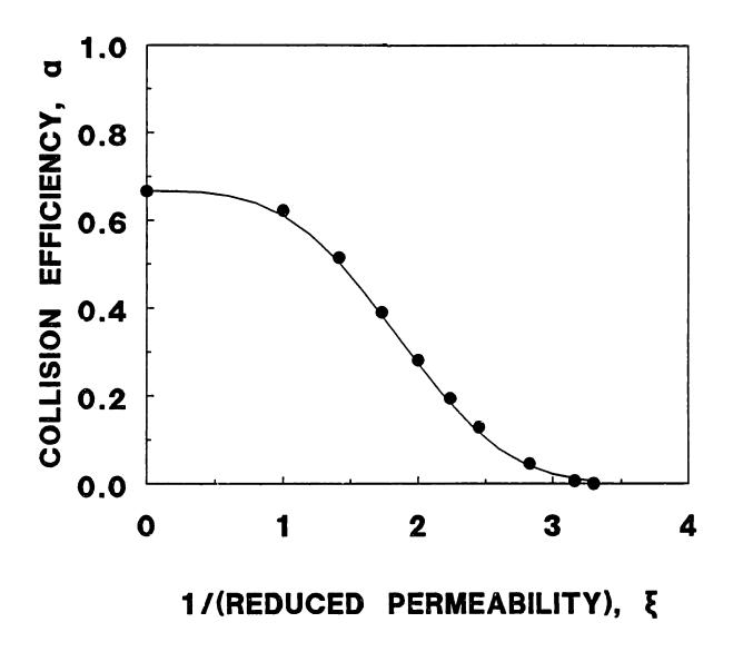
Figure 3-11. Collision efficiency versus the inverse of the normalized floc permeability,  $\xi = a_i/\kappa^{1/2}$  from the calculations of Adler (1981d). The solid line is the prediction of equation (3-36).
