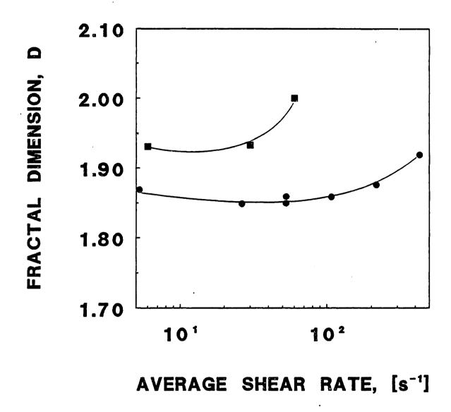
Figure 7-5. Fractal dimension for CRL 1606 flocs versus average fluid shear rate at 50 mg PLH/m². ■ - Couette flow, • - spinner vessel.
