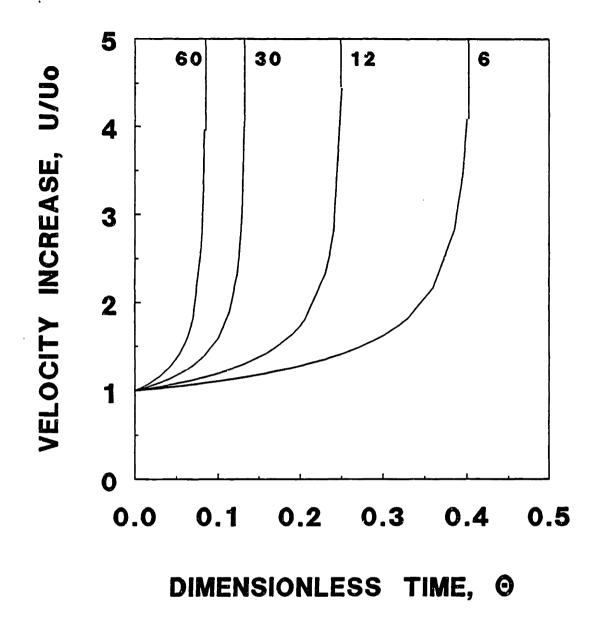
Figure 8-7. Sedimentary velocity enhancement versus dimensionless time predicted by equations (8-10), (8-15) and (8-16) for a polymer dose of 133 mg PLH/m<sup>2</sup>, using the experimental data from chapters 6 and 7. The values of fluid shear rate are shown on the figure.
