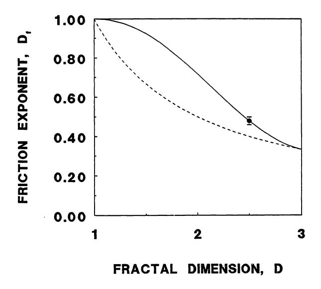
Figure 7-1. Friction exponent,  $D_f$ , calculated by equation (7-7) versus the fractal dimension, D.
