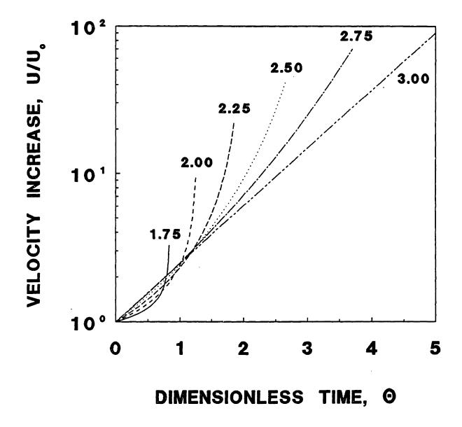
Figure 8-4. Sedimentary velocity enhancement versus dimensionless time for various fractal dimensions, with  $\alpha = 1$ ,  $\dot{\gamma} = 1$  s<sup>-1</sup>. The fractal dimensions are shown on the figure.
