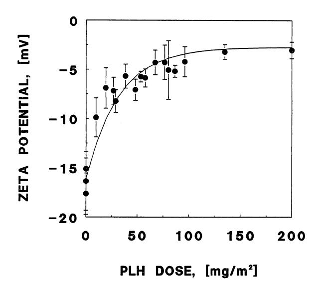
Figure 6-5. Zeta potential of CRL 1606 cells versus poly-L-histidine dose. Solid curve is the best fit regression of the combined equations (6-5) and (6-13) to the data.
