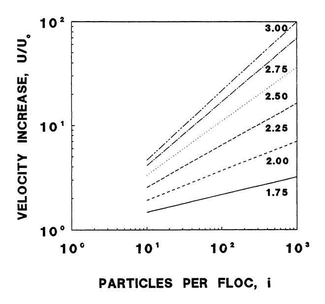
Figure 8-3. Sedimentary velocity enhancement versus the degree of flocculation for various fractal dimensions. The fractal dimensions are shown on the figure.
