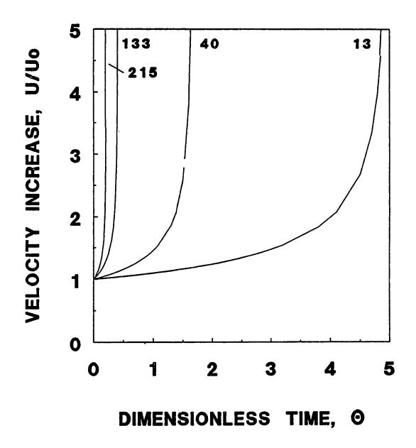
Figure 8-9. Sedimentary velocity enhancement versus dimensionless time predicted by equations (8-10), (8-15) and (8-16) for a shear rate of 6 s<sup>-1</sup>, using the experimental data from chapters 6 and 7. The values of polymer dose in mg/m<sup>2</sup> are shown on the figure.
