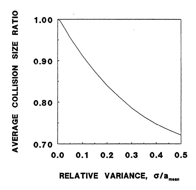
Figure 4-2. Average collision size ratio versus the relative standard deviation about the mean of a normally distributed suspension.
