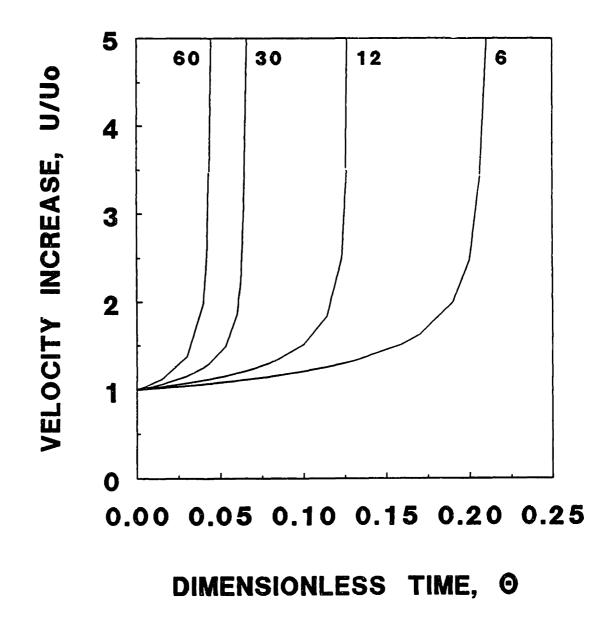
Figure 8-8. Sedimentary velocity enhancement versus dimensionless time predicted by equations (8-10), (8-15) and (8-16) for a polymer dose of 215 mg PLH/m<sup>2</sup>, using the experimental data from chapters 6 and 7. The values of fluid shear rate are shown on the figure.
