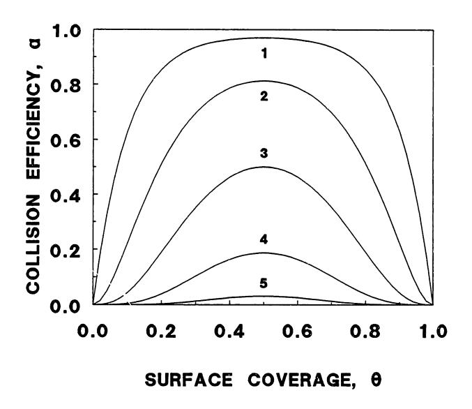
Figure 6-4. Collision efficiency versus fractional surface coverage predicted by equations (6-7) and (6-9) for various m, and n = 5.
