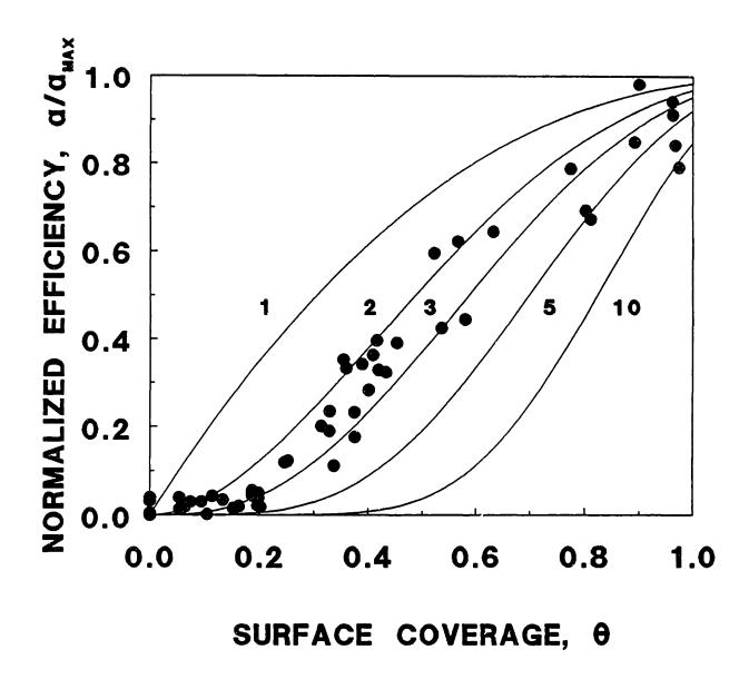
Figure 6-9. Normalized experimental collision efficiency of CRL 1606 cells from Figure 6-7 versus the calculated fractional surface coverage. The solid curves are the theoretical collision efficiencies predicted by equations (6-8) and (6-9) versus fractional surface coverage. The values of n<sub>i</sub> are shown in the figure.
