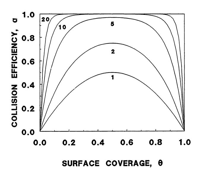
Figure 3-3. Collision efficiency versus fractional surface coverage predicted by the Deason literature model. Numbers indicate the value of  $N_{ij}$ .
