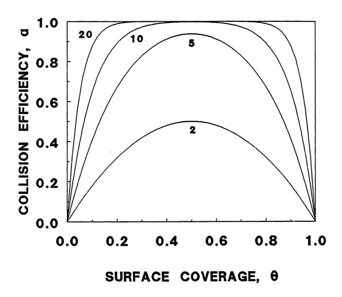
Figure 3-2. Collision efficiency versus fractional surface coverage for the Hogg literature model. Numbers indicate the value of  $(n_i + n_j)$ .
