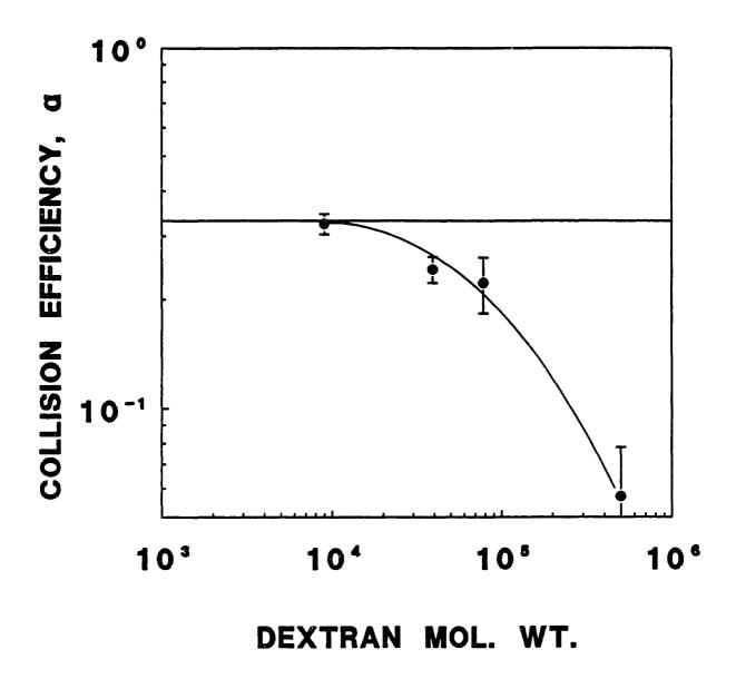
Figure 6-14. Collision efficiency of CRL 1606 cells versus dextran molecular weight at  $\eta = 4.9$  cP, 200 mg PLH/m<sup>2</sup>, shear rate = 30 s<sup>-1</sup>.
