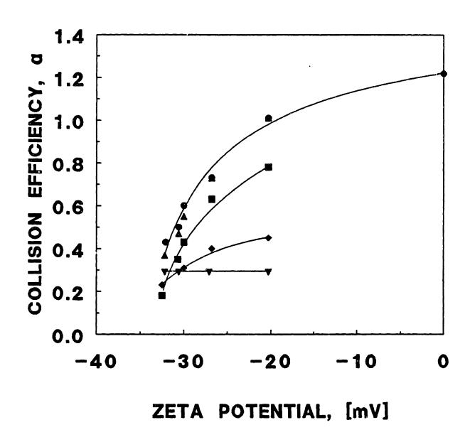
Figure 3-7. Collision efficiency of salt coagulated zinc oxide versus particle zeta potential. Reproduced from Logtenburg and Stein (1985). ● - 400 s<sup>-1</sup>, ▲ - 350 s<sup>-1</sup>, ■ - 300 s<sup>-1</sup>, ◆ - 250 s<sup>-1</sup>, ▼ - 200 s<sup>-1</sup>.
