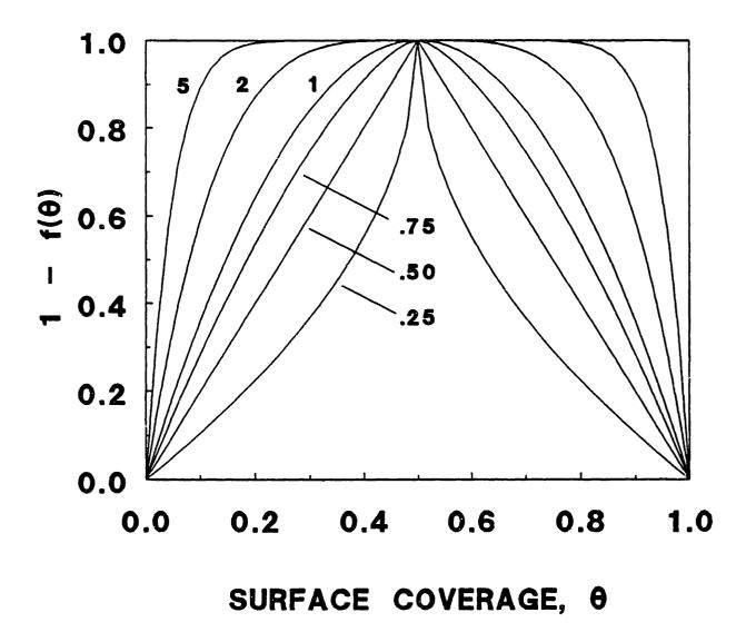
Figure 6-1.  $[1-f(\theta)]$  versus fractional surface coverage for  $z_p = -1$  and varying w. w values are indicated on the figure.
