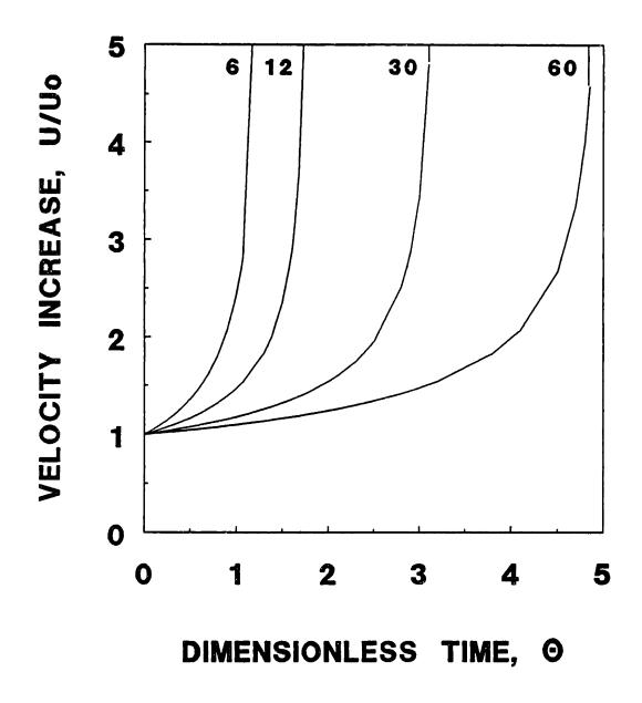
Figure 8-5. Sedimentary velocity enhancement versus dimensionless time predicted by equations (8-10), (8-15) and (8-16) for a polymer dose of 12 mg PLH/m<sup>2</sup>, using the experimental data from chapters 6 and 7. The values of fluid shear rate are shown on the figure.
