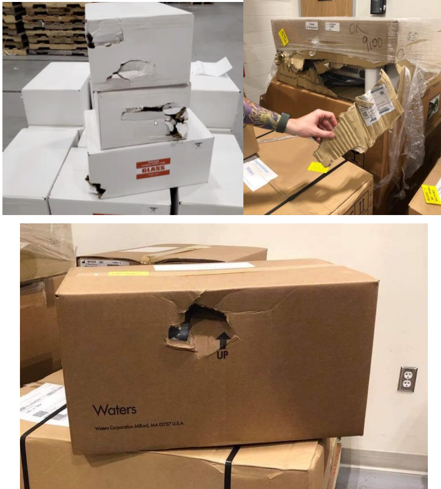
Figure 33: Damage Extended inside without Foam Packaging
