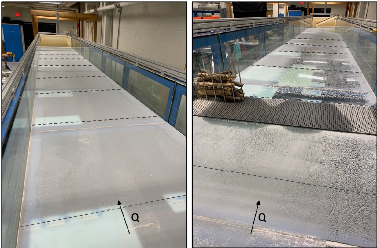
Figure 22: Images of fine sediment deposition on glass bed. On the left is an image of the deposition in the empty flume looking in the streamwise direction. The image on the right is the 0.5 SVF logjam with the resulting deposition, visually quite different from the open bed case. The dashed lines are a meter apart for spatial reference and the arrow represents the flow direction
