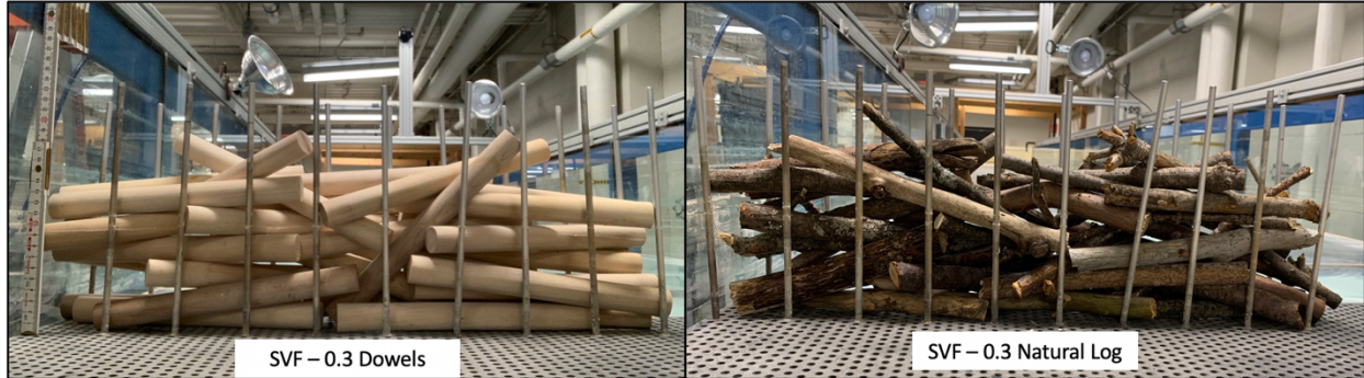
Figure 11: Images of the half width logjams with a SVF of 0.3. On the left using uniform dowels and, on the right, using natural wood logs. The natural logs had a similar but slightly smaller averaged diameter thus 38 logs were used in comparison to 32 dowels. Both images are taken in the flume looking downstream.
