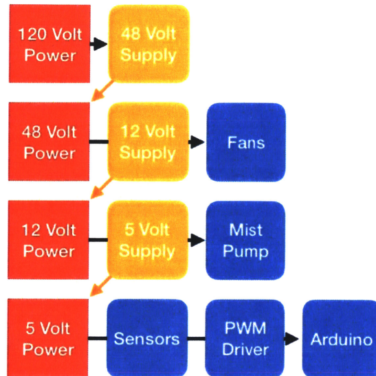
Figure 4.2.1: The above diagram presents a quick overview of the different electrical lines on the system and what each of them powers.
