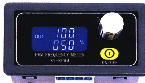
Figure 3.1.2.3: PWM signal generator used to set and monitor fan duty cycle during operation.
