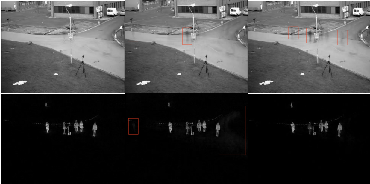
Figure 8-2: Foreground-background separation from video. From left to right: Fast Greedy with rank=3 and Huber loss with \delta = 20 . Standard PCA with rank=1. Principal Component Pursuit (PCP) with \lambda = 0.002 . Both PCA and PCP have visible "shadows" in the foreground that appear as "smudges" in the background. These are less obvious in a still frame but more apparent in a video.
