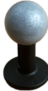
(b) A depiction of a single retro-reflective marker used tracked by the motion capture system.
