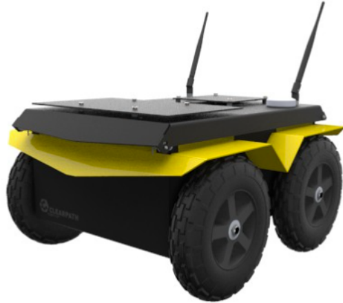
Figure 2-1: A depiction of the Jackal Unmanned Ground Vehicle (UGV) from Clearpath Robotics, which was used as a mobile robot base for this iteration of the system.
