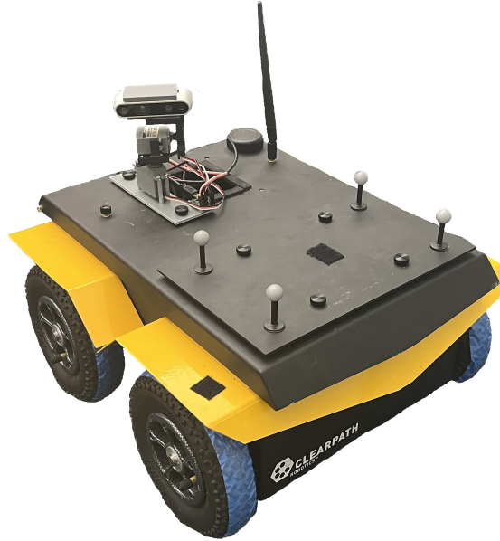
Figure 2-6: The above figure depicts the object-based navigation system described in this chapter in its fully assembled state.
