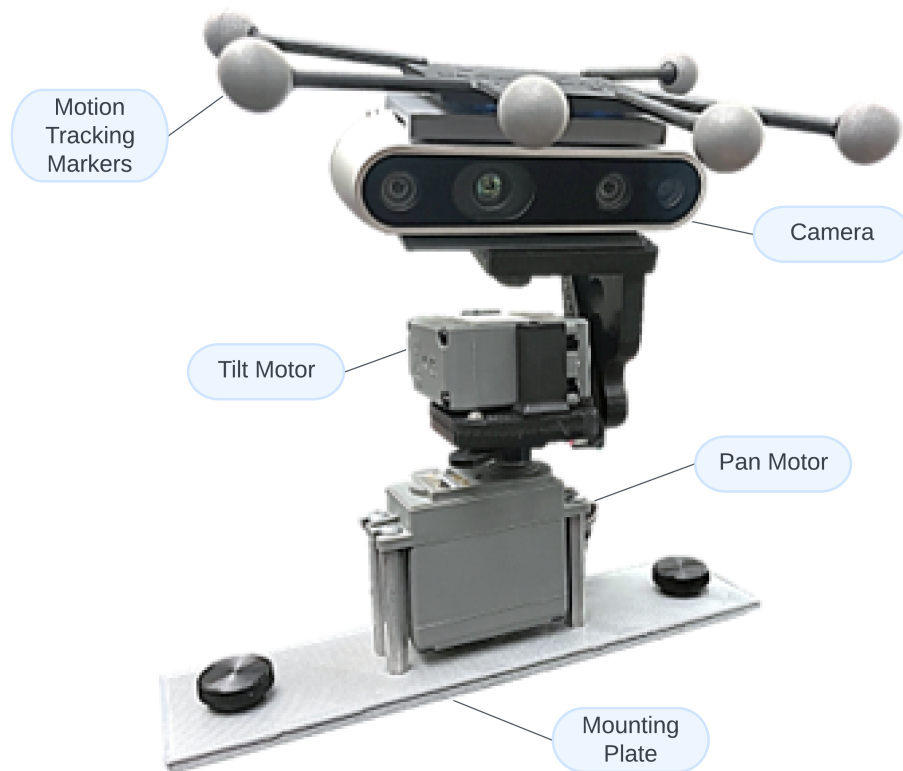
Figure 2-2: The above figure shows a labeled depiction of the visual servoing module. Two goBilda Servo Motors are stacked in a pan-tilt configuration, with a mounted RGB-D camera. The camera is topped with a set of retro-reflective markers for motion tracking, and the whole assembly is affixed directly to the Jackal using 3D-printed mounting plate.
