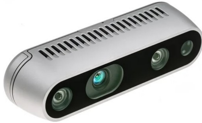
Figure 2-5: The Intel RealSense D435 RGB-D camera, shown here, is a stereoscopic depth camera that was mounted on top of the pan-tilt module. The visual data from the camera was used for object detection and 6-DOF pose estimation.
