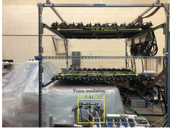
Figure 4.6: The GAPS functional prototype demonstrated the successful operation of all flight systems using \sim 10\% of the Si(Li) modules and TOF paddles of the full flight payload. Photo courtesy of Mengjiao Xiao.
