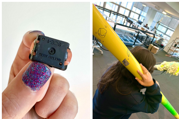
Figure 79 (Left) Bone conduction transducer. Photo: Nicole L'Huillier. (Right) Kimy listening to the tube. Photo: Nicole L'Huillier.
