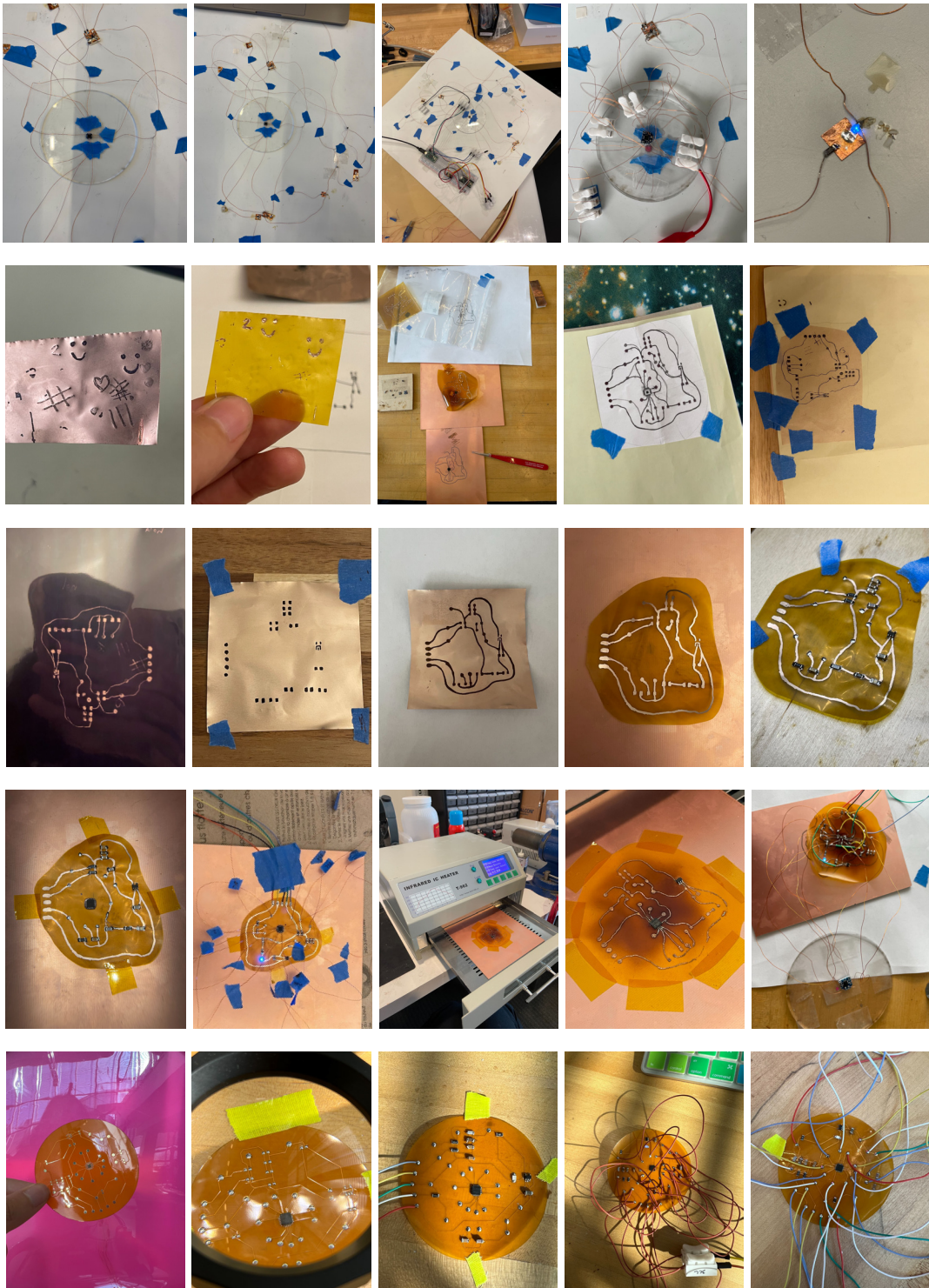
Figure 59 Soft sensor process. From initial tests and designs to the final flexible printed circuit board (PCB).
