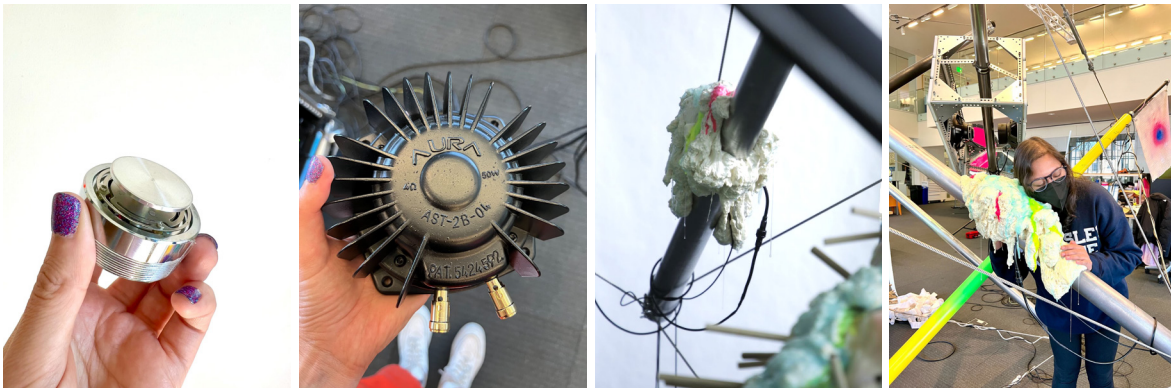
Figure 78 (Left) Tactile transducer 25W. Photo: Nicole L'Huillier. (Center Left) Low-frequency shaker transducer 50W. Photo: Nicole L'Huillier. (Center Right) Transducers in installation. Photo: Nicole L'Huillier. (Right) Kimy perceiving the vibrations with her head and hands. Photo: Nicole L'Huillier.
