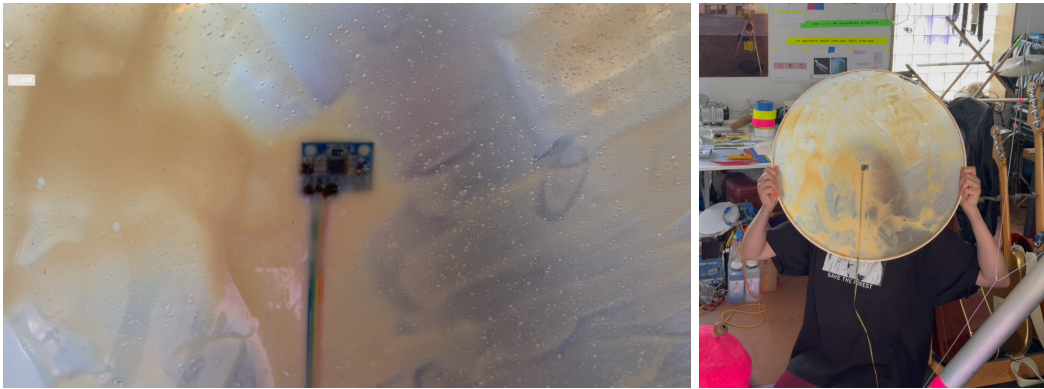
Figure 53 Latex/natural rubber experiments. Membrane with accelerometer MPU6050.
