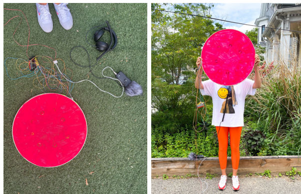
Figure 51 Eight-channel natural rubber pigmented membrane with piezoelectric sensors.
