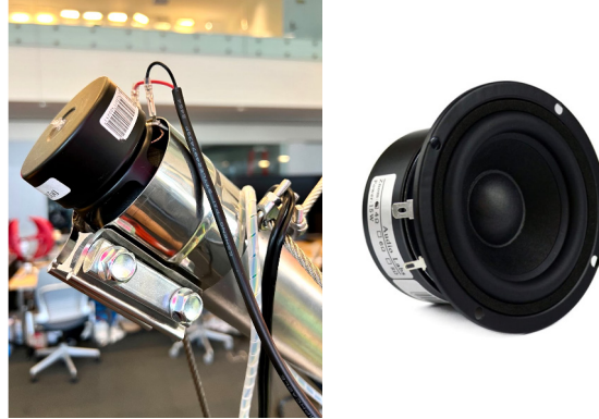
Figure 77 (Left) Speaker attached to the tube. Photo: Nicole L'Huillier. (Right) Picture of the speaker. Photo: Facmogu, model A18021.
